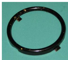
The locking lever engages the internal tab shown here (l-r) from the back of the ring and the front. The external tab fits a slot in the finger wheel between the O-1 position to the right of the finger stop.
