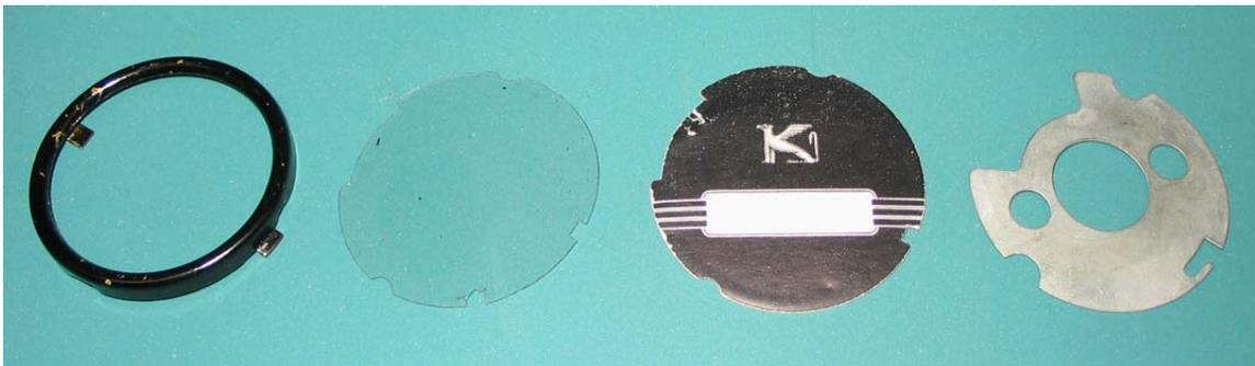
The dial card is assembled as shown left to right; the notch in the four o'clock position of the window and card fits a tab (shown in the left picture at the top in the two o'clock position) and insures that the card is positioned correctly when installed on the dial.
