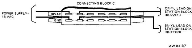
Figure 10: Connecting Details, Button and Buzzer Signaling
