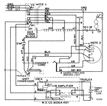
NORTH ELECTRIC CO. TELEPHONE SET MODIFIED FOR USE WITH W.E. 6030A KEY
