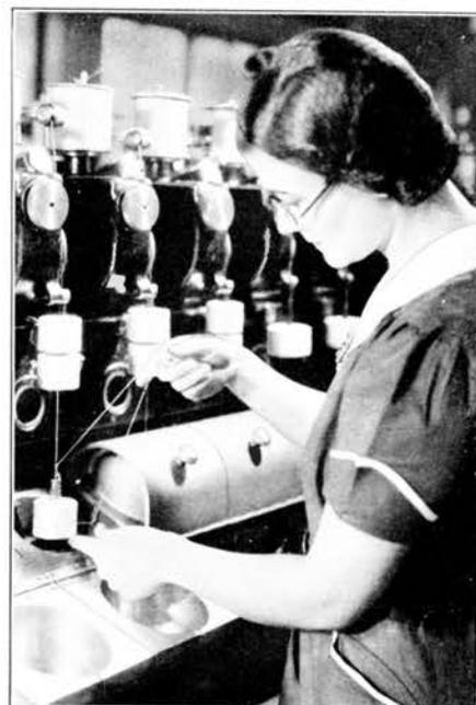
*Silk is wrapped around fine copper wire in a serving machine pictured above. The operator is adjusting the silk band to assure perfect coverage of the wire.*
