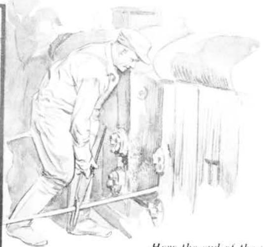
*Here the end of the red hot copper rod is being placed between the revolving rolls, reducing its size and increasing its length.*
