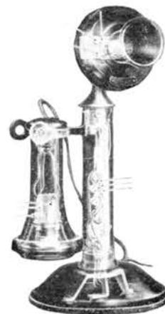
*Nickel is sometimes used as a protective coating on the parts of the transmitter indicated by the three upper arrows and as plating on connectors in the receiver and for springs in the body of the instrument.*
