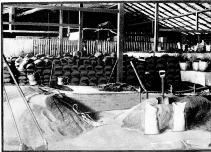
After the tin has been separated from the gravel it is put in bags to go to the smelters from which it comes out as the tin of commerce.
