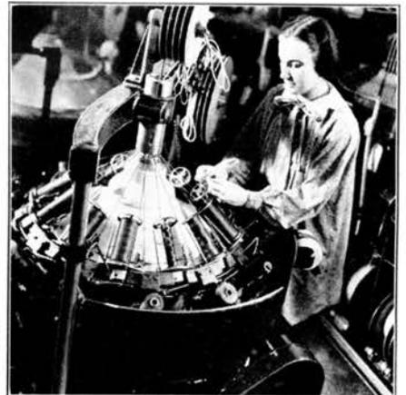
*Cotton braid protects many types of telephone cords. As the insulated wires or cords come up through the center of this machine, spindles of cotton thread move round and round braiding on the protective layers.*
