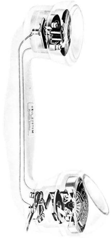
*A phantom view of the telephone handset handle—the transmitter and the receiver. As illustrated and explained on the previous page, the entire case is molded of phenol plastic compound. There are a dozen additional different insulating and moisture-proofing materials in your handset: Cotton, rubber, flax (paper), phenol fibre, clay, talc, silk, wax, hemp (paper) and shellac.*
