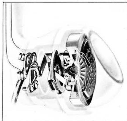
*A phantom view of your handset transmitter. The dome-shaped dark mass in the center is the carbon granules. There is a paper seal between the diaphragm and the electrode to prevent the carbon granules from leaking out.*
