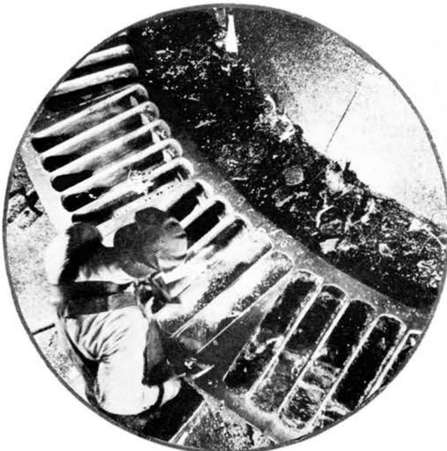
*Mechanically activated casting wheels mold the lead into silvery "pigs" ready to begin its final, vital job of protecting the nation's speechways.*
