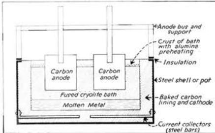
*This sectional view of an aluminum furnace or "pot" shows the arrangement of the parts and materials described in the text.*
