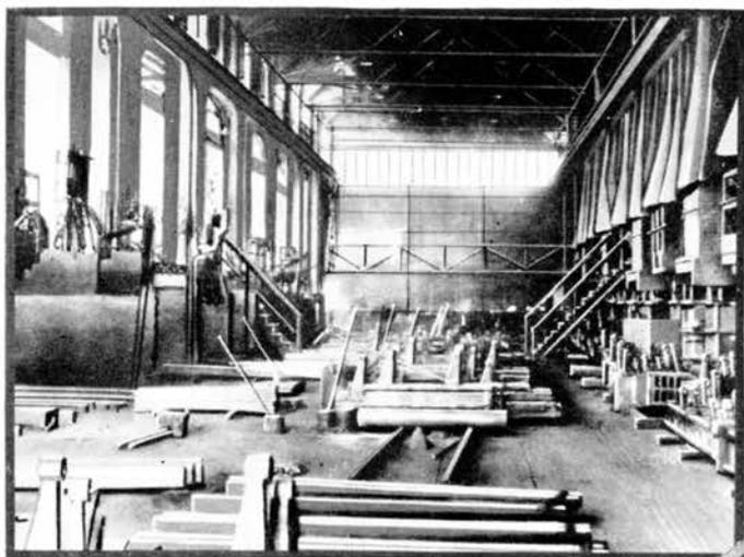
*A section of the casting floor in a brass foundry with furnace, exhausters and other equipment.*
