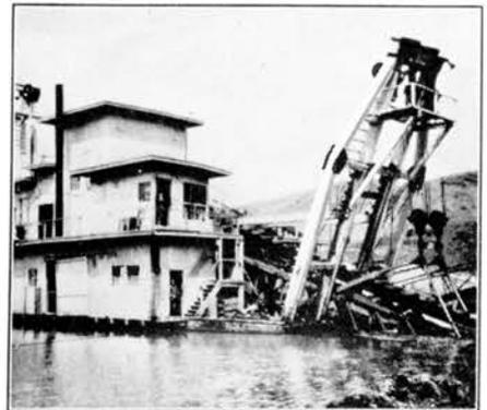
*Dredges are now the chief means by which alluvial gold is recovered. Here is a large unit at work in Oregon.*
