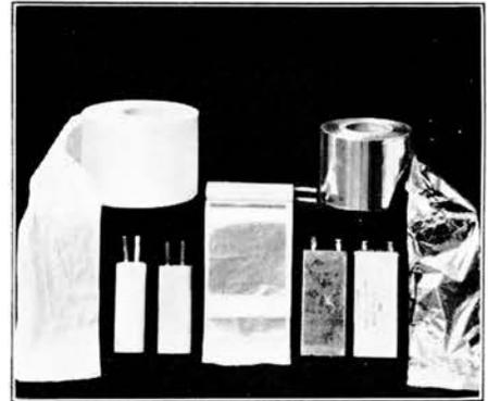
*Aluminum foil is used in the manufacture of condensers. At the top are rolls of insulating paper and foil; in the center a condenser unit, slightly unrolled; while in the lower view are (left to right) a condenser unit before and after baking and waving; a potted condenser before cleaning and painting—the unit having been inserted in a can which was then filled with asphalt compound; and at the extreme right the finished product.*
