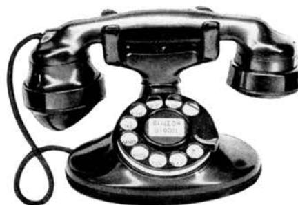
*Alloy steel is used in the magnet and diaphragm of your handset telephone. The cradle and base are of zinc alloy, while the base plate, covered with leather, is of iron.*
