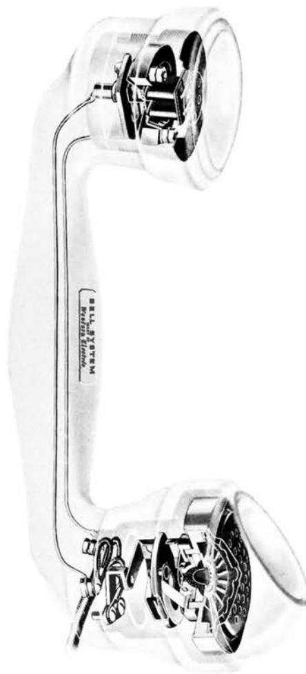
*A phantom view of your handset telephone. Practically all of the metal parts are made of various alloys that serve best each part for its particular job of giving telephone service. Some of the details of the transmitter and receiver are explained in later chapters.*
