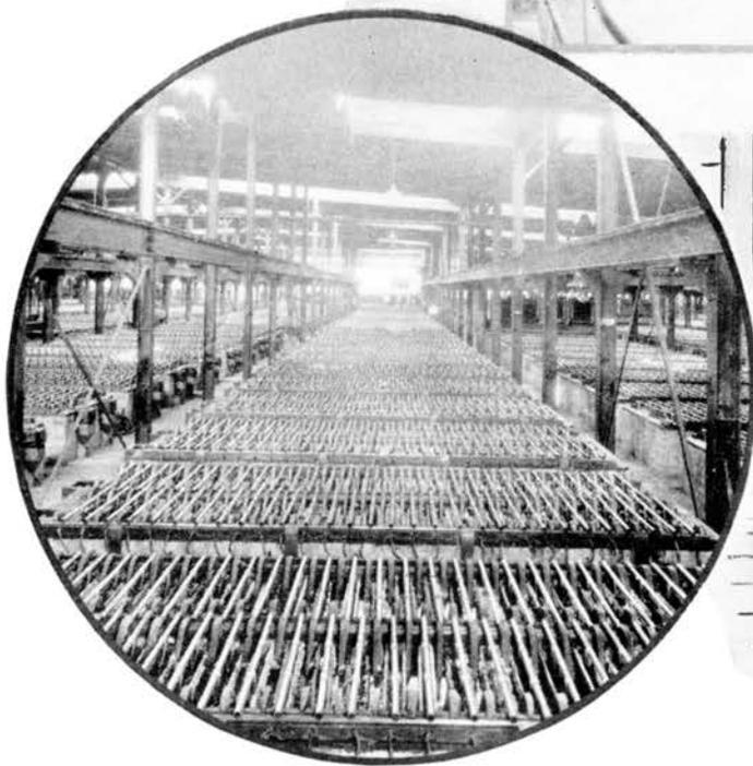
*Six acres of cells for the production of pure electrolytic nickel.*
