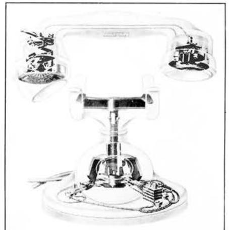
*The cord emerging from the handle of this telephone set, those seen inside and those connecting cords (see text) coming from the base of the stand are covered with an insulation made of cotton.*
