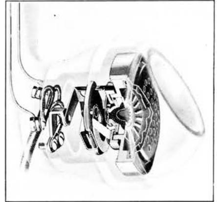
*The carbon grains in your telephone are in the small receptacle just in front of the aluminum alloy diaphragm of the telephone transmitter, phantom view of which is shown above.*
