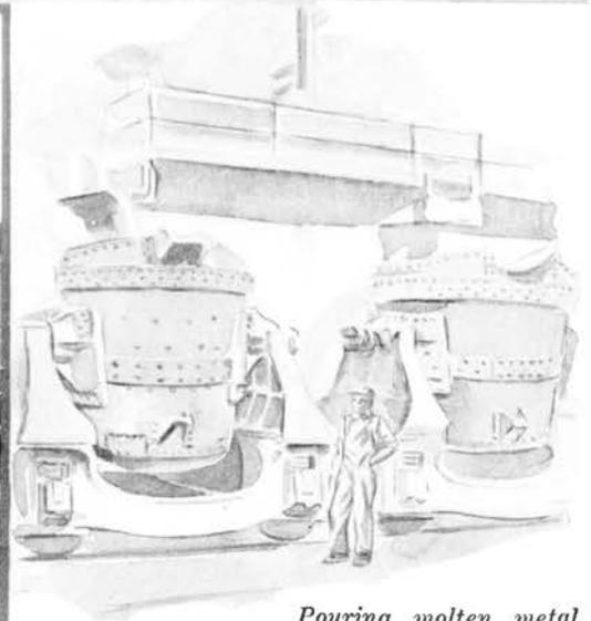
*Pouring molten metal from a furnace into a kettle carried on its own car.*
