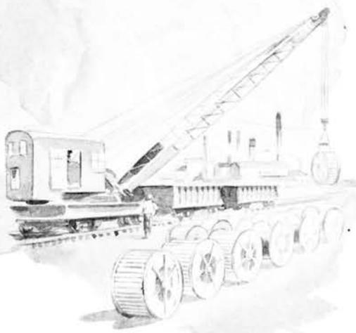
This crane locomotive, operated by an electric storage battery, handles heavy cable reels.
