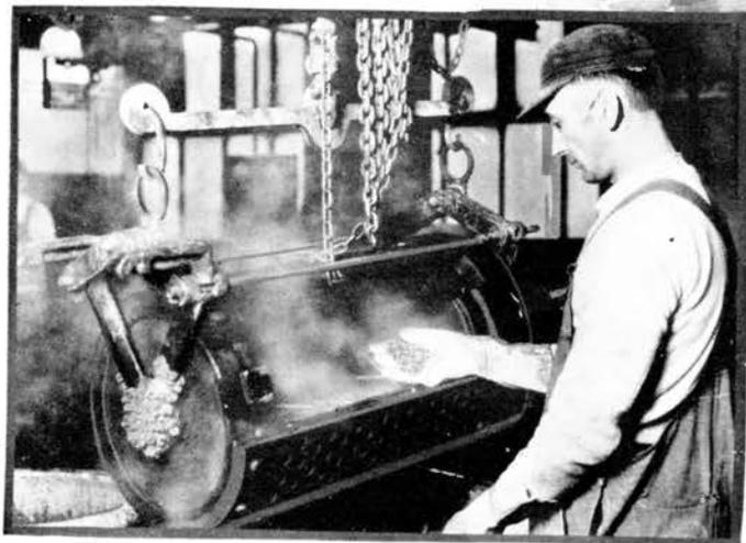
*Zinc is the great protector of iron and steel products, which it shields from rusting from the effects of air and water, with a protective coating called galvanizing.*
