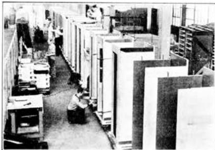
*In another wood-working shop scientifically prepared woods are used to construct telephone booths.*
