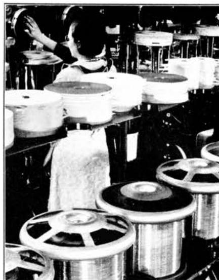
*A row of paper insulating machines. The shiny copper wire shown on the spools in front of these insulators is wrapped with insulating paper much like one would tape a baseball bat, except that very close limits must be maintained.*
