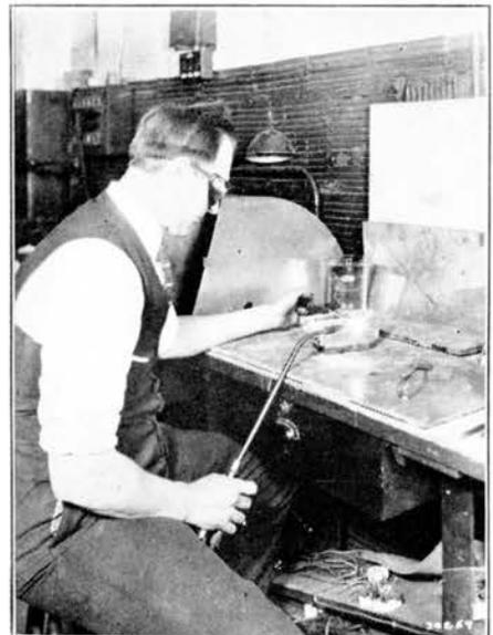
*Preparation of platinum alloys for vacuum tube filaments.*
