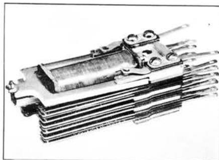
*Nickel is part of the alloy used in the relay illustrated above, a type employed by the tens of thousands in telephone systems. Nickel is used in the winding wire, contact springs, magnetic structure and finish of the relay.*
