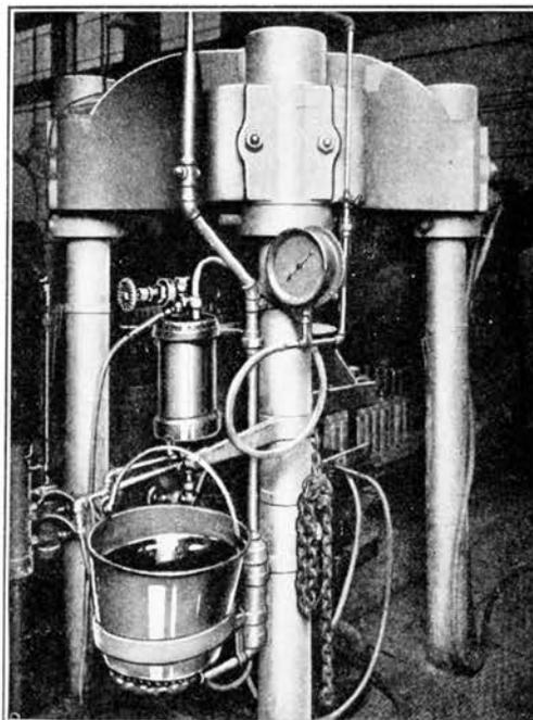
*In this press, thin hollow lead piping is filled with rosin to make easy-to-use rosin core solder.*
