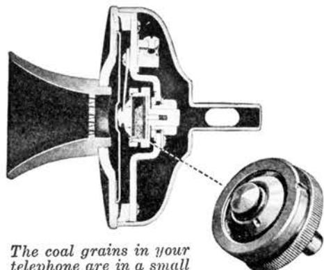
*The coal grains in your telephone are in a small receptacle just behind the aluminum diaphragm of the telephone transmitter.*
