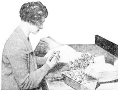
*Nickel is used as a finish to insure resistance to atmospheric effects on many of the parts used in telephone apparatus.*
