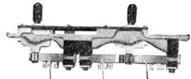
*Nickel silver is used in the mechanism of the keys the switchboard operator manipulates to listen-in to learn what number is wanted and also to "ring" the called subscriber.*
