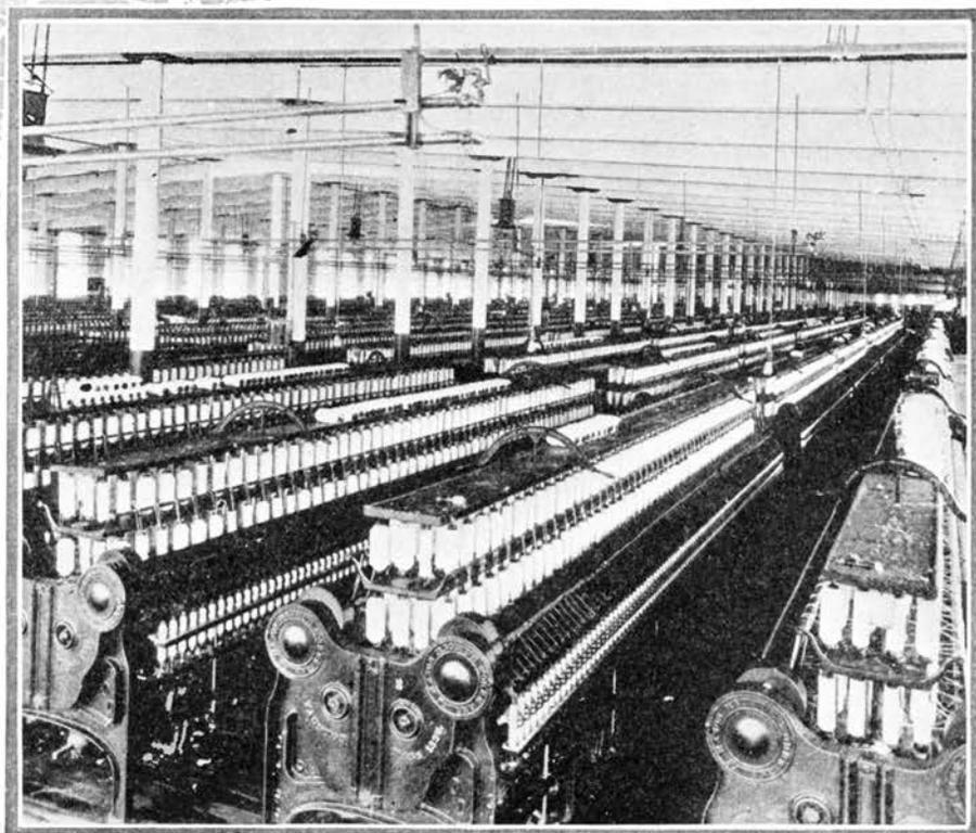
*Spinning—After being carded, the fibres are stretched on drawing frames, twisted and finally wound on bobbins which spin them into thread for weaving.*
