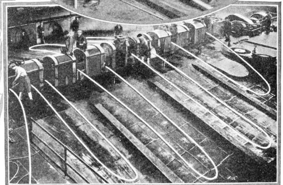
*Each pass through the rolls reduces the thickness of the copper and increases the length, so that now the bar, which was originally 54 inches long and 4 inches square, has become 1200 feet long and only  $\frac{1}{4}$  inch thick.*
