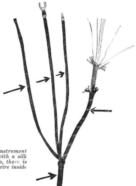
*The cords which reach from your telephone instrument to the box on the wall or desk are covered with a silk braid to insulate and protect the wires. Too, there is a silk insulation wrapped around the copper wire inside the cord.*
