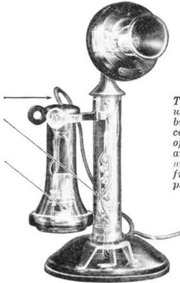
*The arrows show where silk is braided on to the cords and wires of your telephone and on the cord which extends from your telephone to the box on the wall.*
