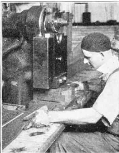
From long narrow strips of soft rubber, machines punch out pieces, shaped like half of the receiver rolled out flat.
