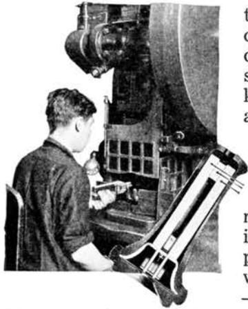
*The three pieces of iron forming the receiver magnet of your telephone are welded by electric heat to form one solid piece. By making the iron all one piece a better electrical pathway is obtained than by hammering or swaging.*
