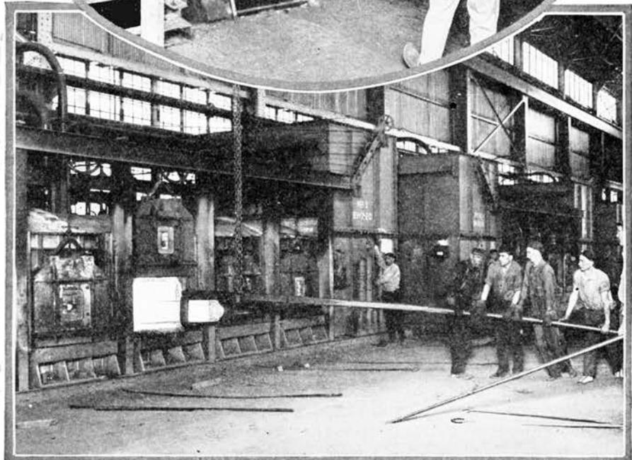
*Forging a 2-ton nickel ingot with a steam hammer.*
