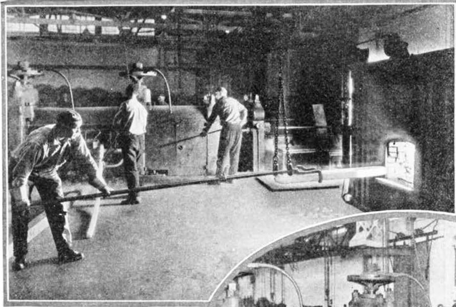
*Below—A few more passes through the rolls and the copper bar has become a long thick, snake-like rod of copper.*
