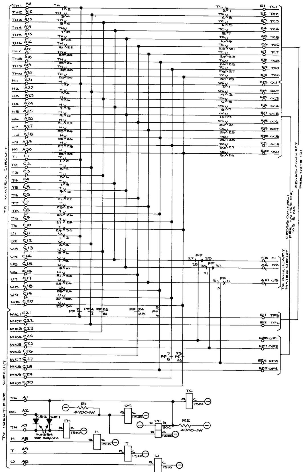
Figure 6. Matrix Reduction Circuit.
