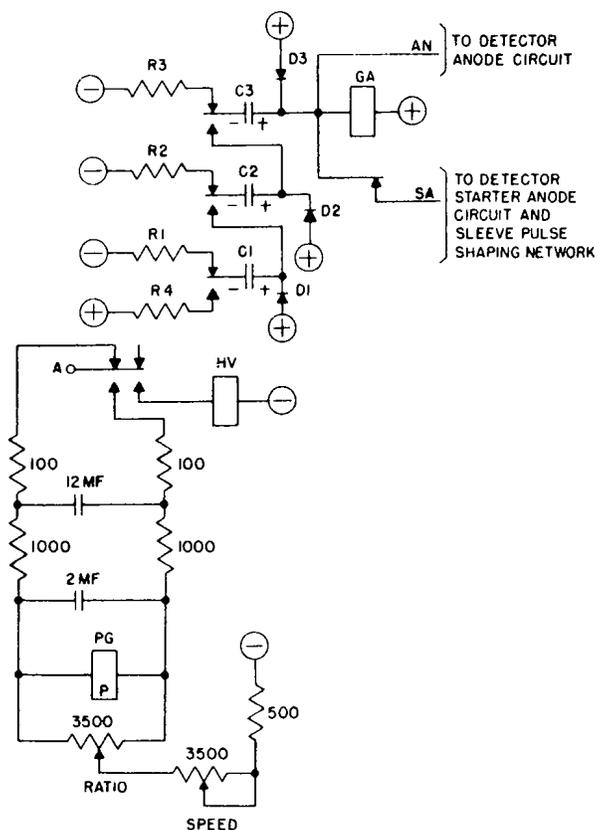
Figure 2. High-Voltage Pulse Generator
