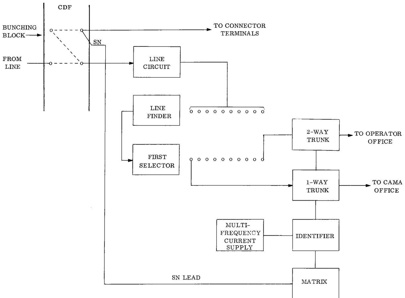
Figure 1. Typical Application of Identifier in CAMA Tributary Office.
