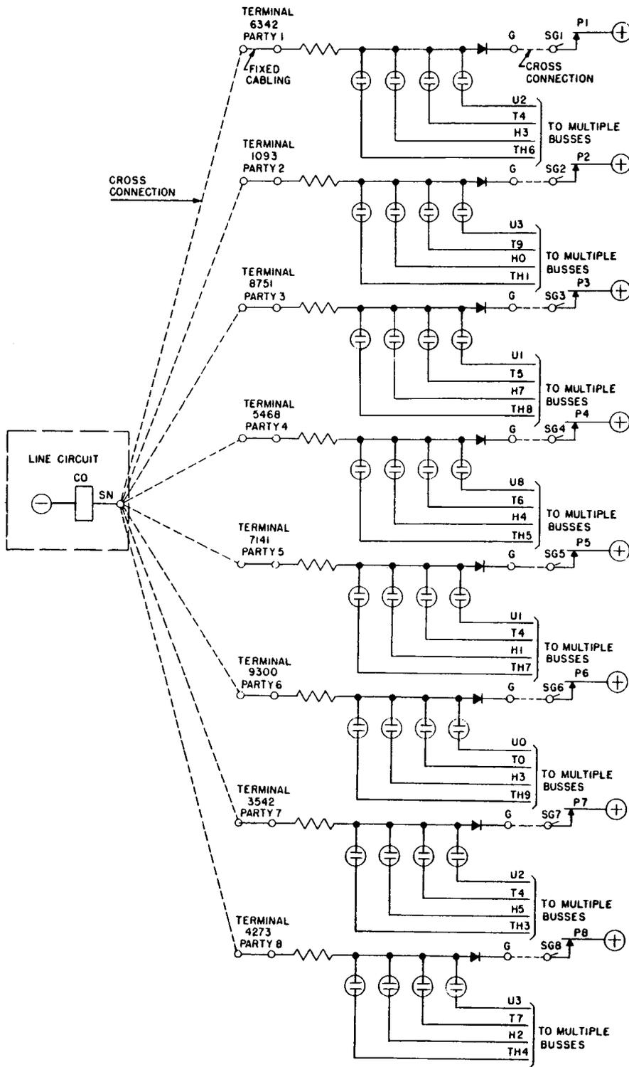
Figure 4. Terminal-Per-Station Gating Arrangement
