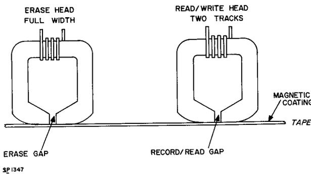
Figure 1. Recorder Head Configuration.
