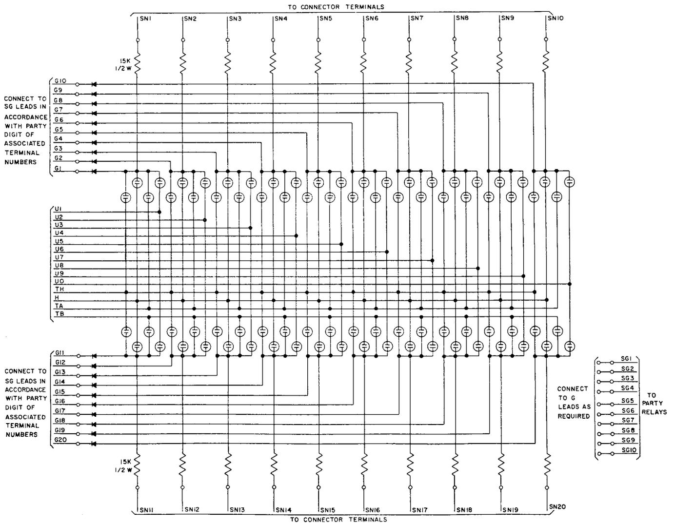
Figure 3. Terminal-Per-Station Matrix Arrangement
