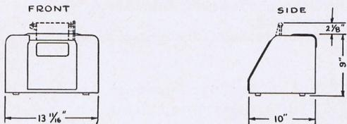
Tear-off type CB11-11 or CA11-11. Also available with winder of upright type (shown by dotted lines) as Models CB12-11 or CA12-11. The upright winder can be extended 9" from the top, making an overall height of 17 3/4".
