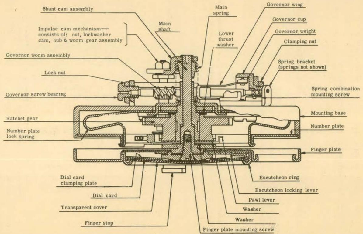
Fig. 11. Cross section of type 51 dial.
