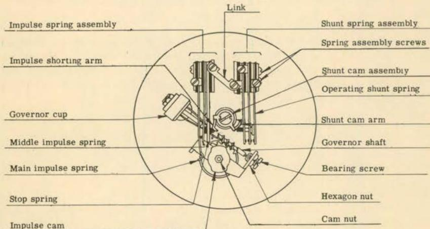
Fig. 2. External details of standard dial (rear view).
