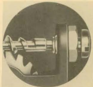
Fig. 4. Worm gear and governor worm assembly.
