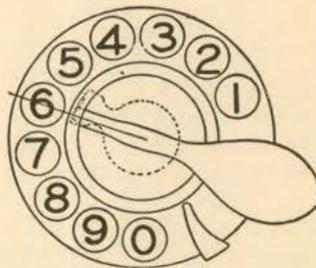
Fig. 9. Escutcheon ring locked.
