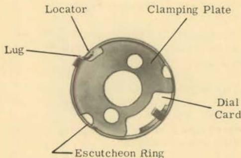
Fig. 7. Rear view of dial escutcheon assembly.
