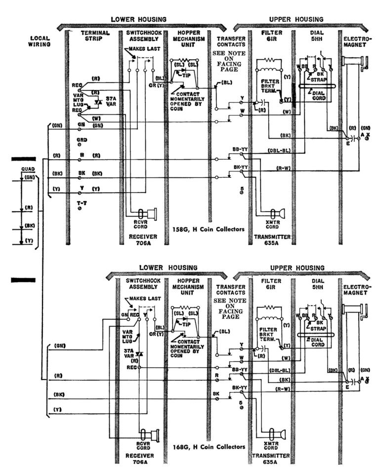
Fig. 1 — Circuit Diagram for Use with 634BA and 684BA Induction Coil Type Subscriber Sets
