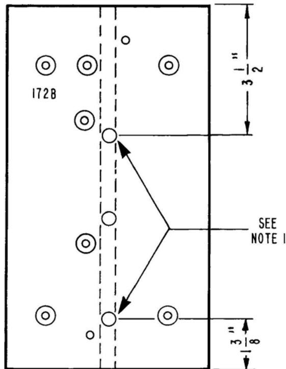
**Note:** These 3/8-inch holes are not provided in the 172A, but may be drilled in the field to accommodate type 554, 556, or 558 telephone sets. The top hole is usually provided for the type 558 set, and the bottom hole for types 554 and 556 sets.
