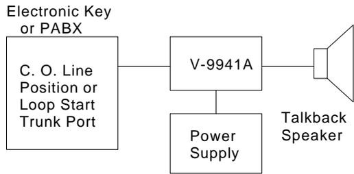
**Figure 1 - Typical Loop Start Trunk Installation**
