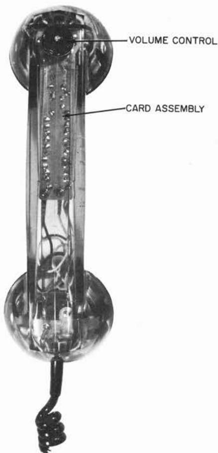
Figure 2. Type 820 Handset (Top View).
