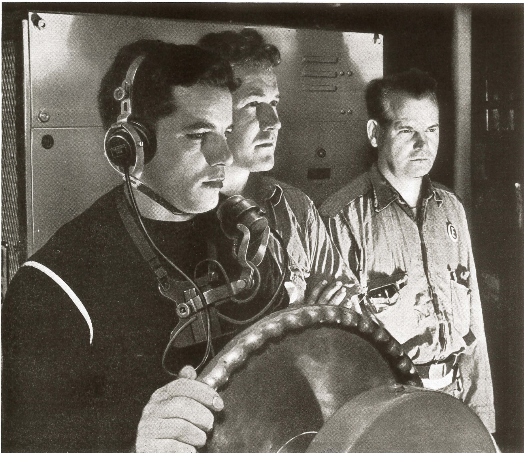
EMERGENCY STEERING STATION on U. S. battleship. The helmsman gets steering instructions over a battle telephone. The two other men are intently watching their gauges.
