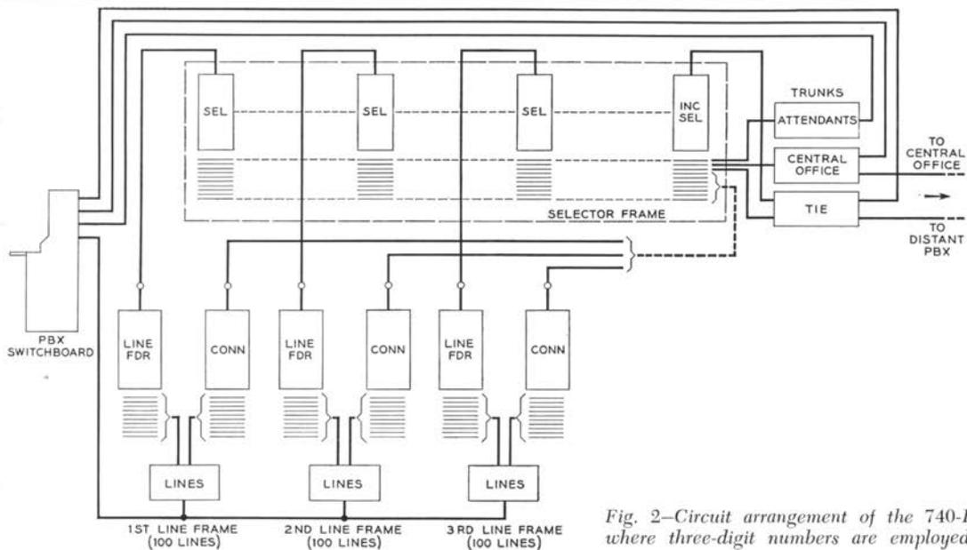
Fig. 2—Circuit arrangement of the 740-E where three-digit numbers are employed
