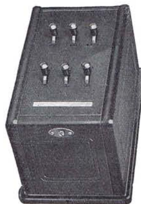
In order that outside service may be given to the two-wire intra-house stations a small transfer key box is provided at a master key station
