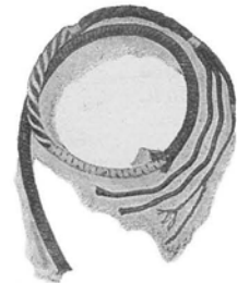
Construction of Moisture-proofed Tinsel Telephone Cords
