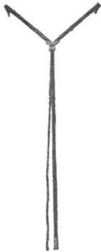
End Section with Spreaders Extended No. 3 Line Pole
