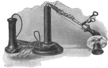
Showing Method of Removing Working Parts
