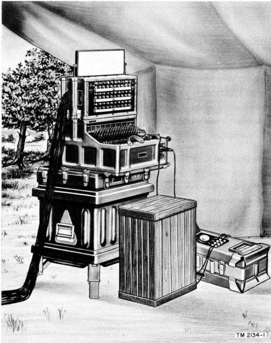
*Figure 1. Manual Telephone Switchboard SB-86/P, set up for use.*
