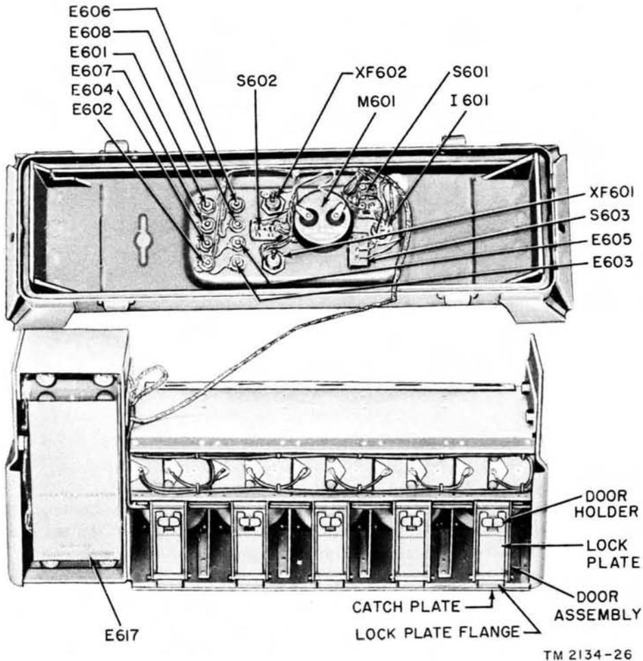
Figure 34. Power Supply PP-990/G, location of parts.
