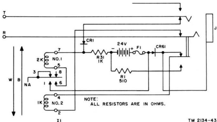
Figure 24. Common battery signaling trunk line circuit, simplified schematic.
