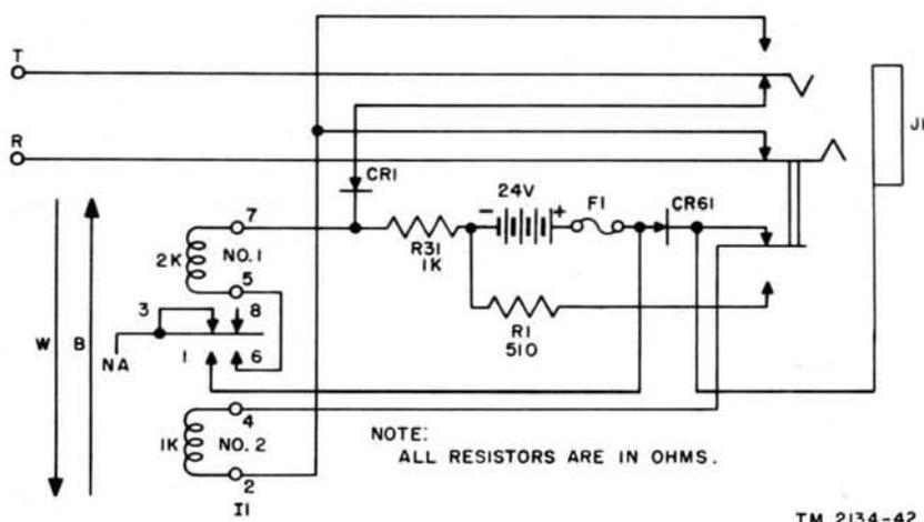
Figure 23. Common battery signaling line circuit, simplified schematic.
