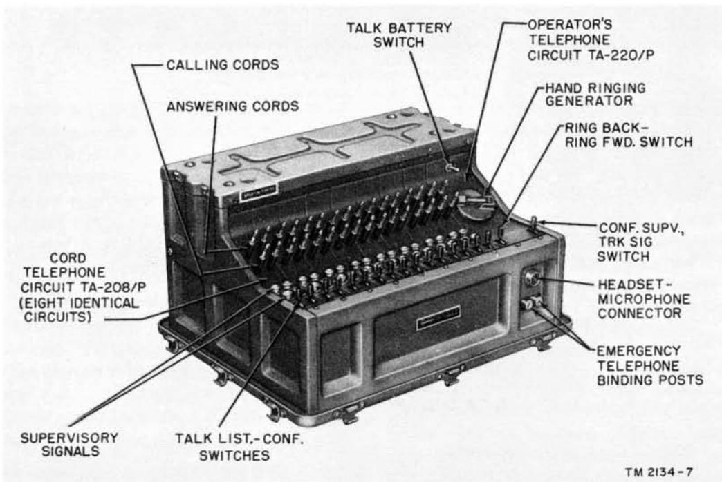
Figure 6. Manual Telephone Switchboard Section SB-248/P (keyshelf section).
