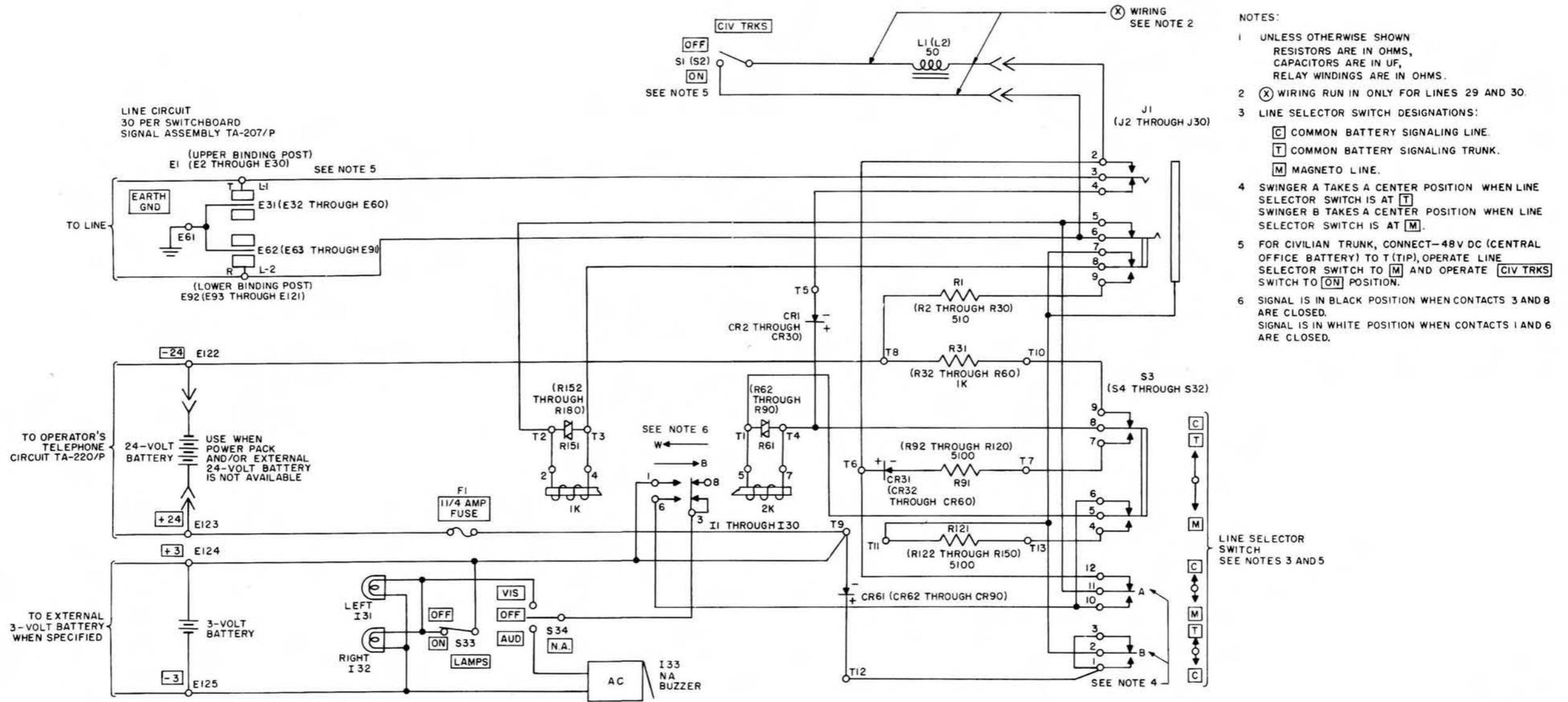
Figure 40. Switchboard Signal Assembly TA-207/P, schematic diagram.
