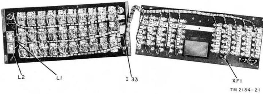
Figure 26. Switchboard Signal Assembly TA-207/P, dismantled for maintenance.
