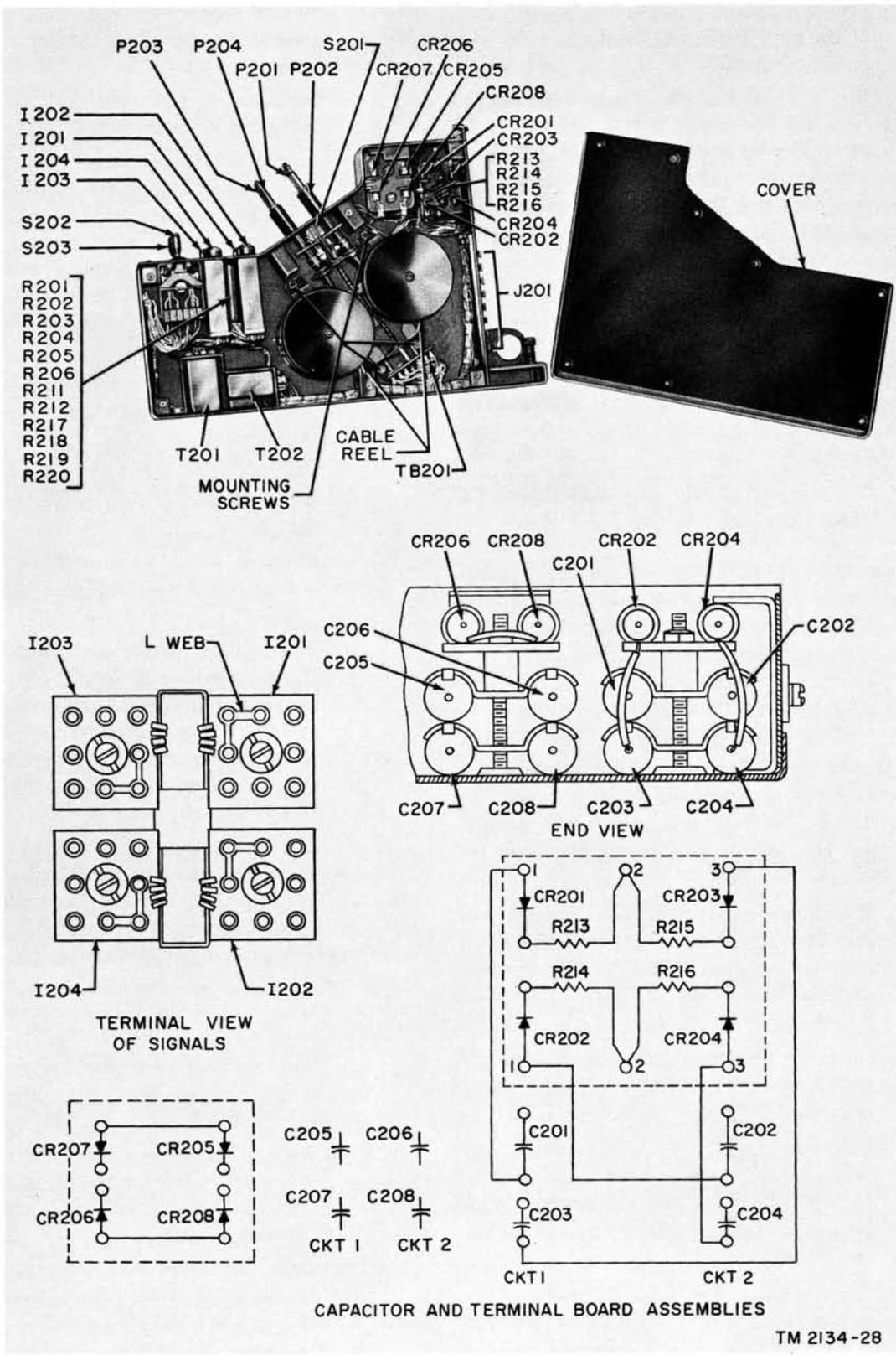
Figure 30. Cord Telephone Circuit TA-208/P, location of parts.
