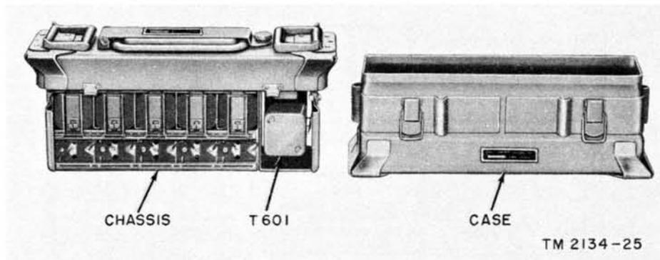
Figure 16. Power Supply PP-990/G, case removed for battery installation.
