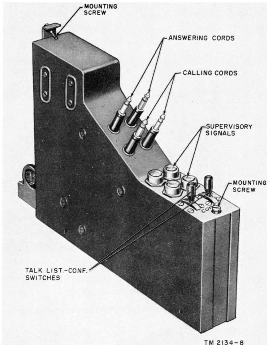
Figure 7. Cord Telephone Circuit TA-208/P (cord pack).
