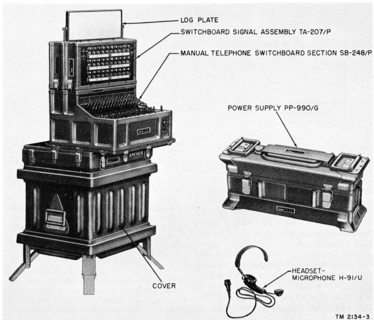
Figure 3. Manual Telephone Switchboard SB-80/P, components less power cords and spare parts.
