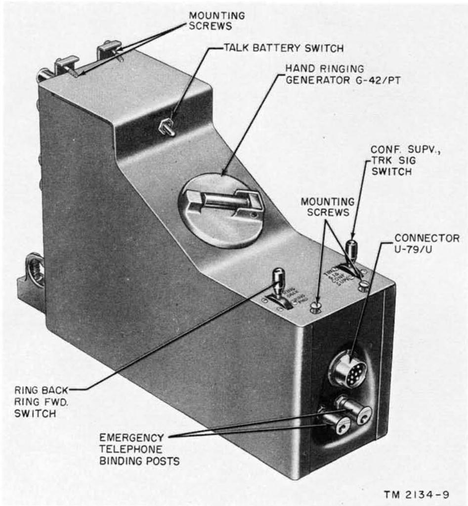
Figure 8. Operator's Telephone Circuit TA-220/P (operator's pack).
