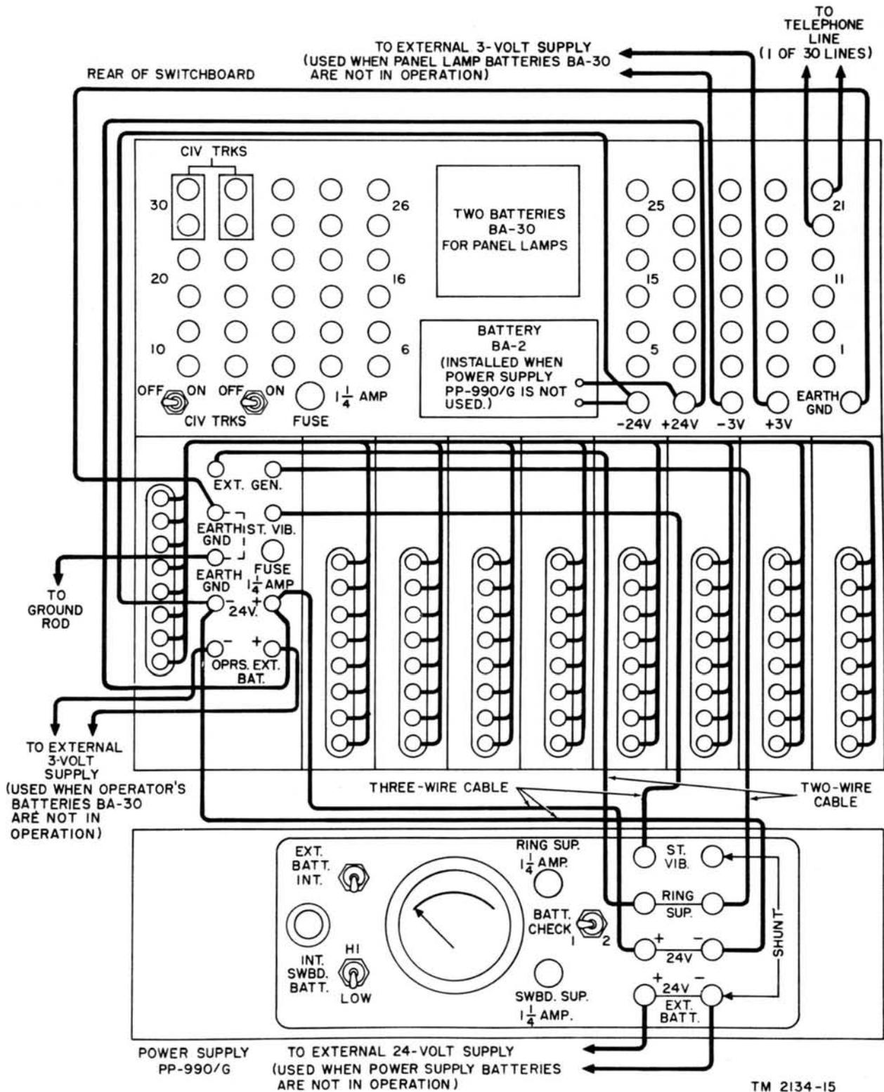
Figure 18. Manual Telephone Switchboard SB-86/P, cording diagram.
