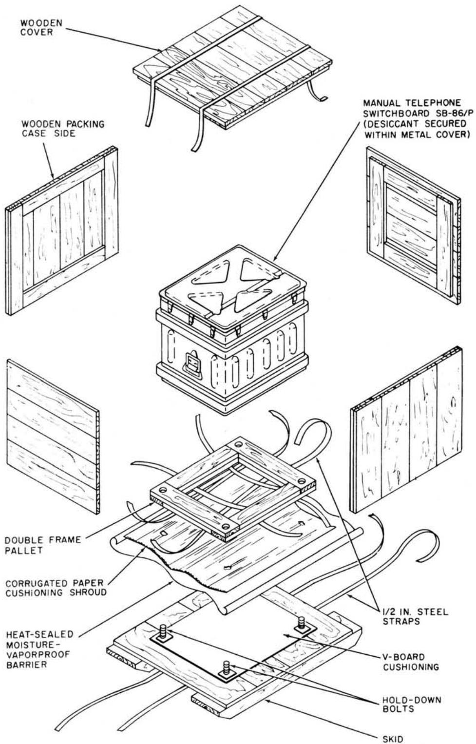
Figure 13. Manual Telephone Switchboard SB-86/P, packaging diagram for export shipping.
