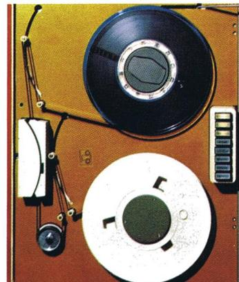
To add CAMA equipment to serve over 40,000 lines requires adding only one 27-inch rack, eight feet high. Records for 1,000 completed calls can be stored on only nine feet of magnetic tape (a reel holds up to 2400 feet). Electronic circuitry minimizes maintenance. Centralized automatic message accounting relieves burden on toll office ticketing facilities.
