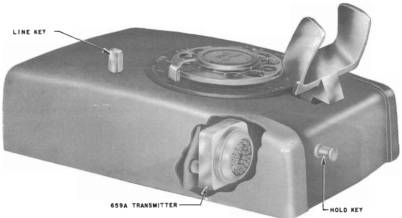
Fig. 5 — 558C/D Telephone Set Modified to Include 659A Transmitter Unit
