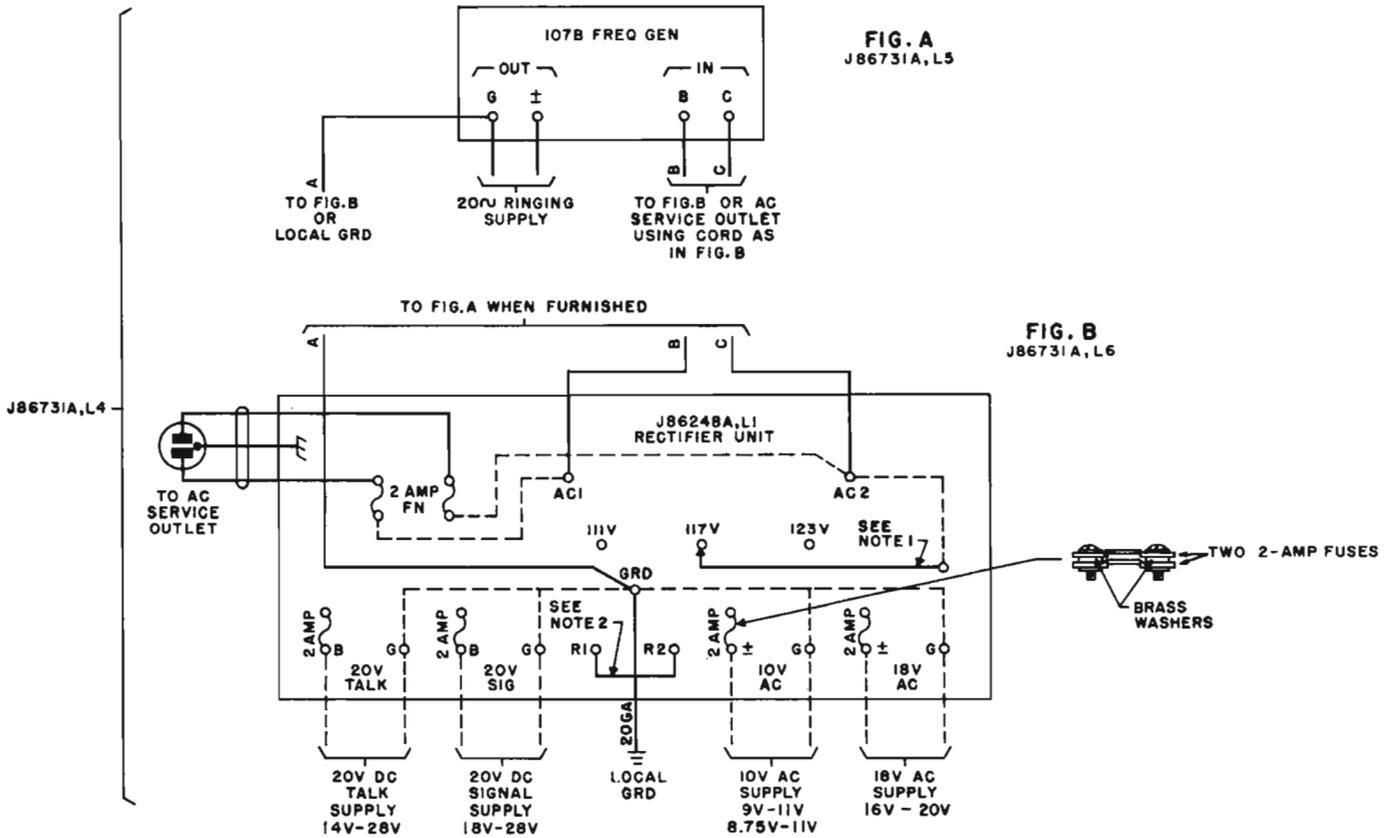
**Note 1:** Connect to 111V, 117V, or 123V, depending on ac service voltage range.
