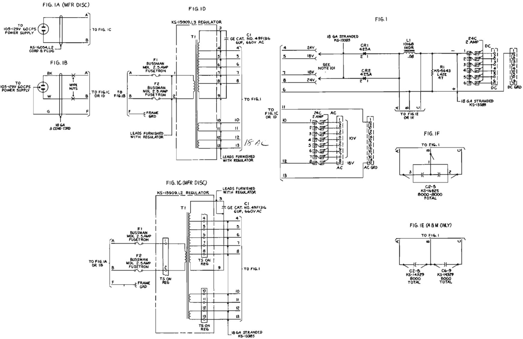
**Note 1:** When rectifier is used with key telephone equipment, connect 24V taps. When used with PBX equipment, connect 18V taps.
