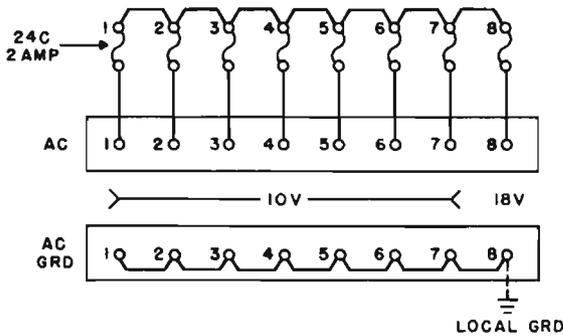
Note: Connect the BK lead to the B terminal. Connect the G and W leads to the 18V terminal when used with PBX equipment, and to the 24V terminal when used with key tel equipment.
