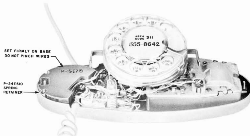
Fig. 6 - Location of Cold Cathode Tube in 701B Telephone Set
