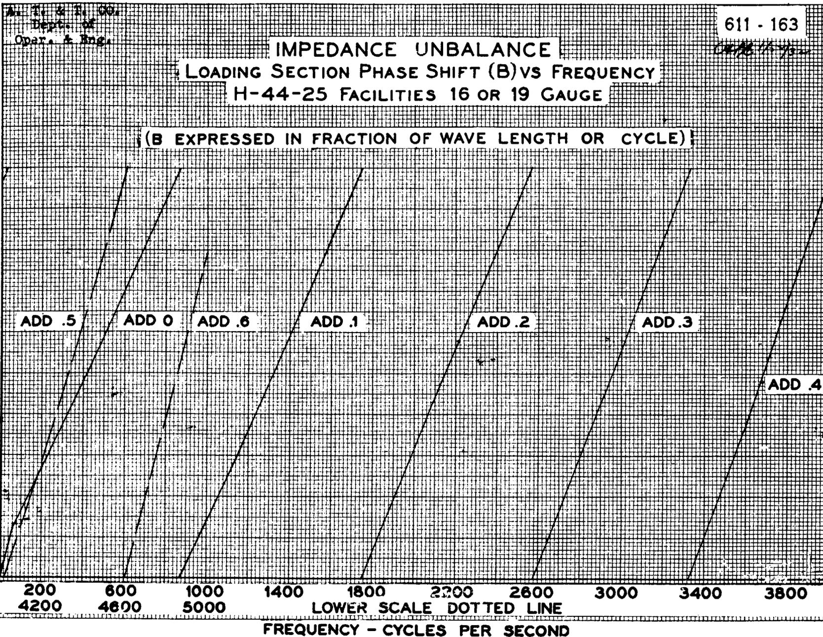
PHASE SHIFT (°) PER LOAD SECTION - OUT ON PHANTOM, RETURN ON SIDE
