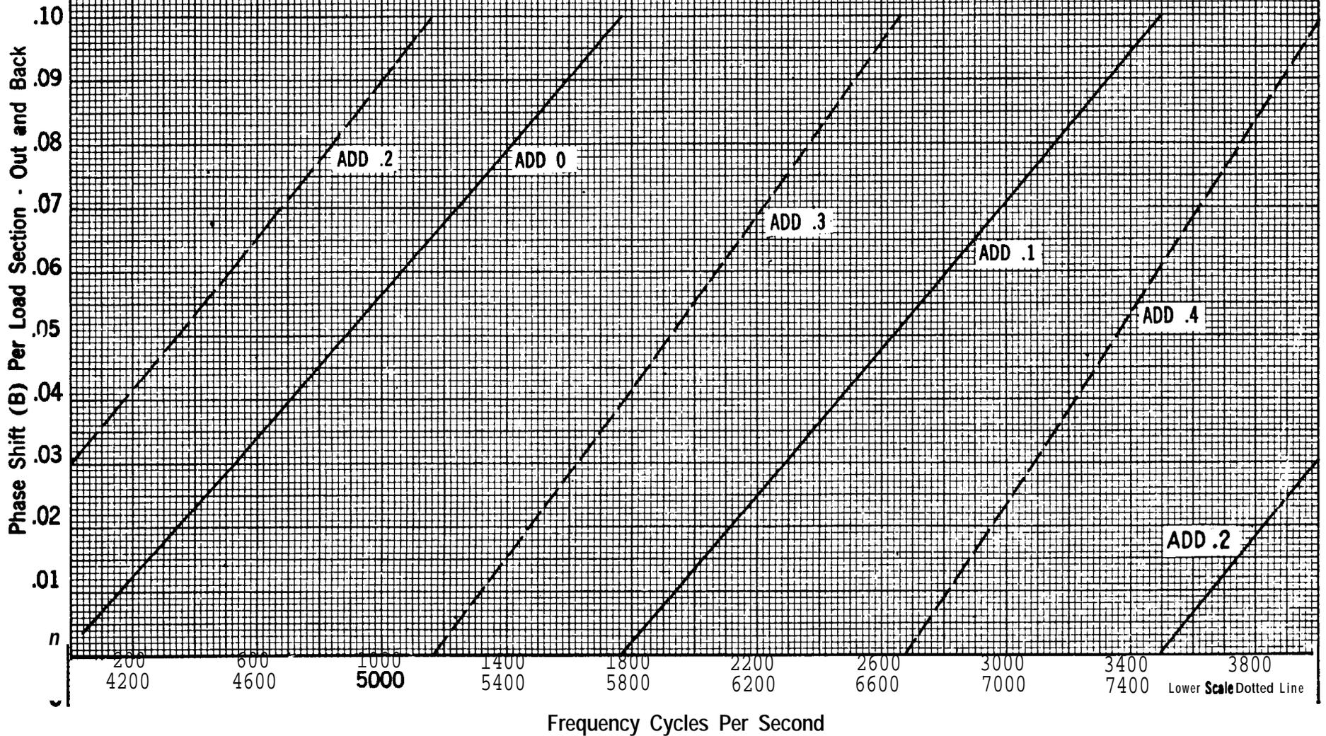
PHASE SHIFT (B) PER LOAD SECTION - OUT ON PHANTOM, RETURN ON SIDE
