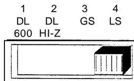
1. Dry Loop 600 Ohms, used for input from paging port of PBX or from microphone
