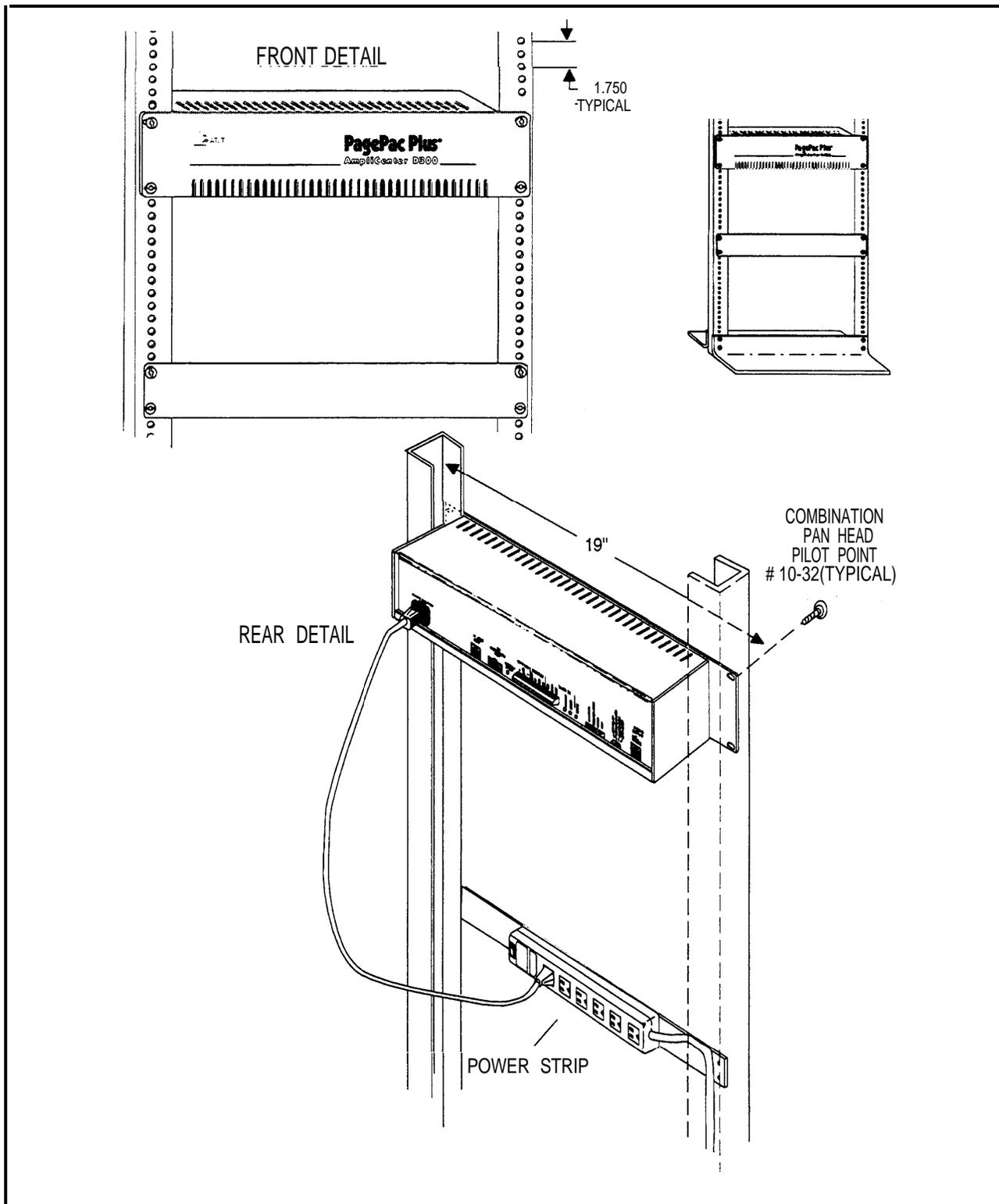
Figure 3-4. Rack Mounted Hardware
