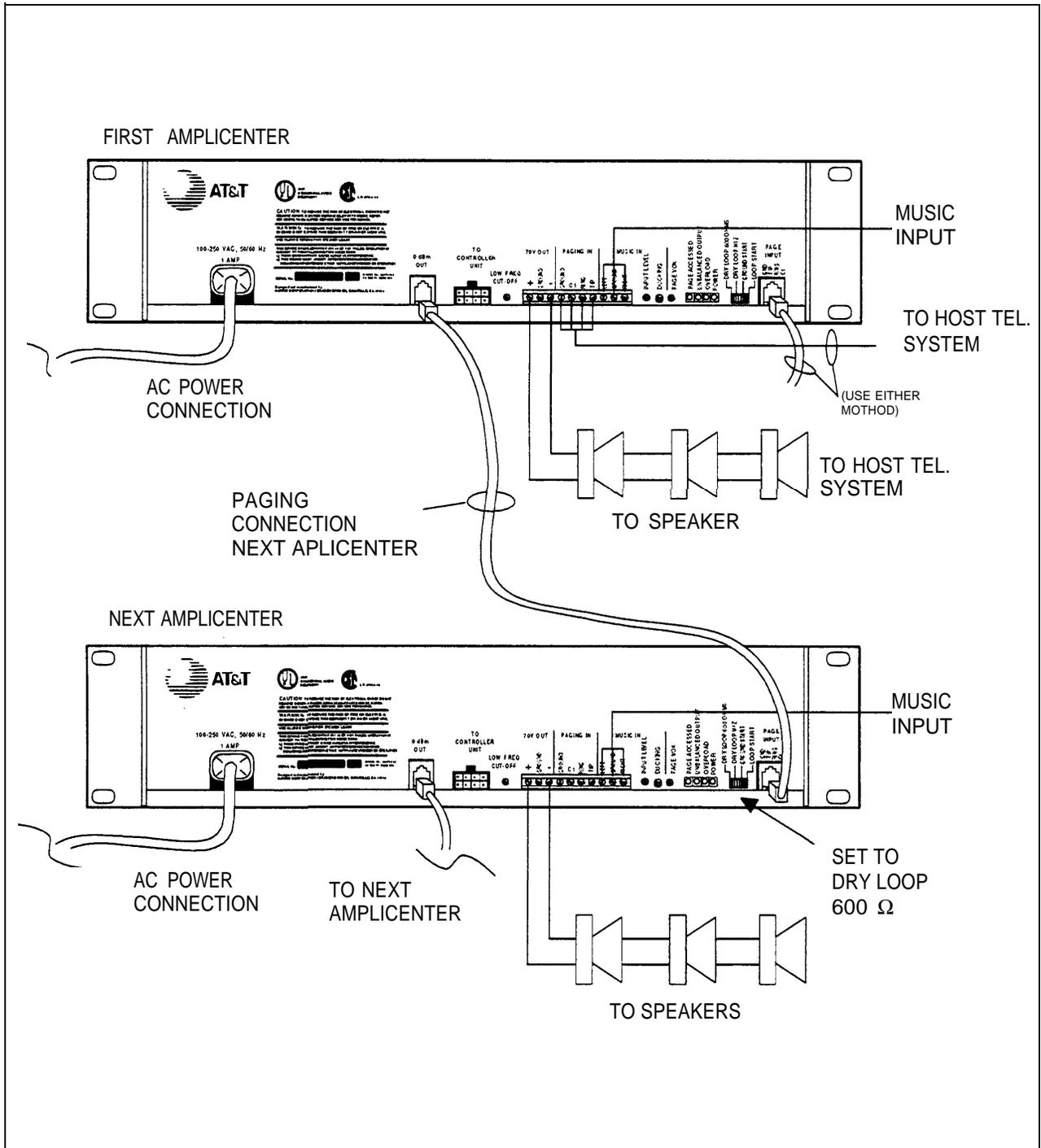
Figure 3-2. Series AmpliCenters, without Controller
