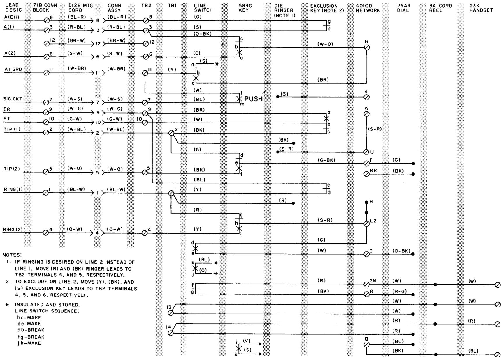
◆Fig. 2—1751C and D Telephone Set Connections With 25A3 (MD) Dial◆
