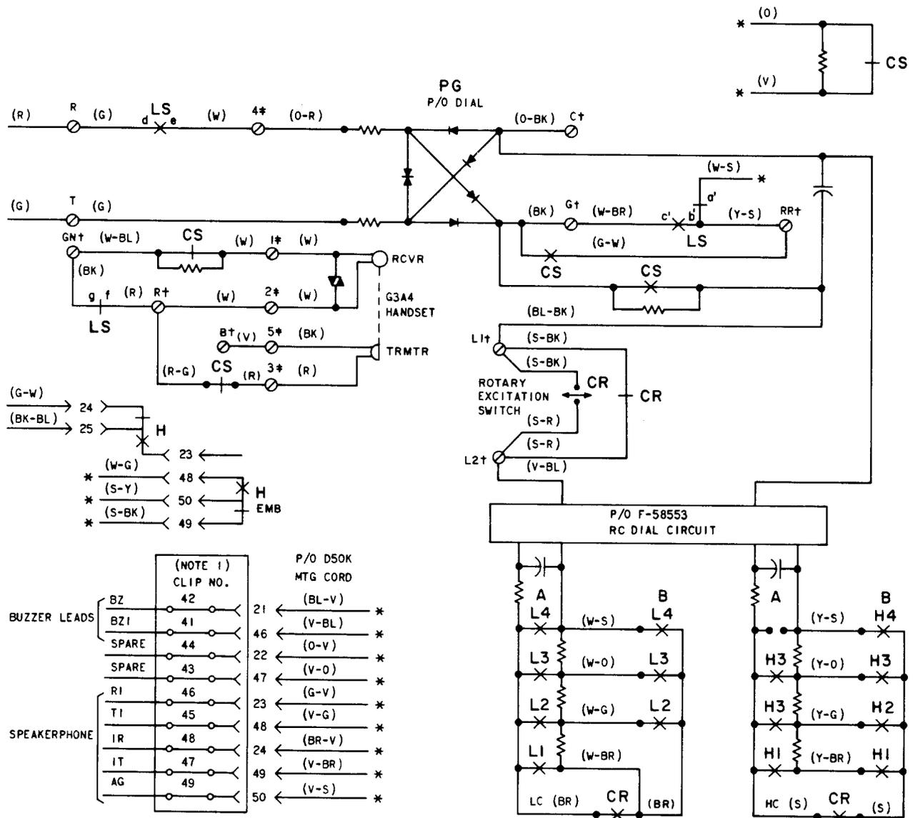
Fig. 5—F-58555 Telephone Set Connections (Sheet 2 of 2)
