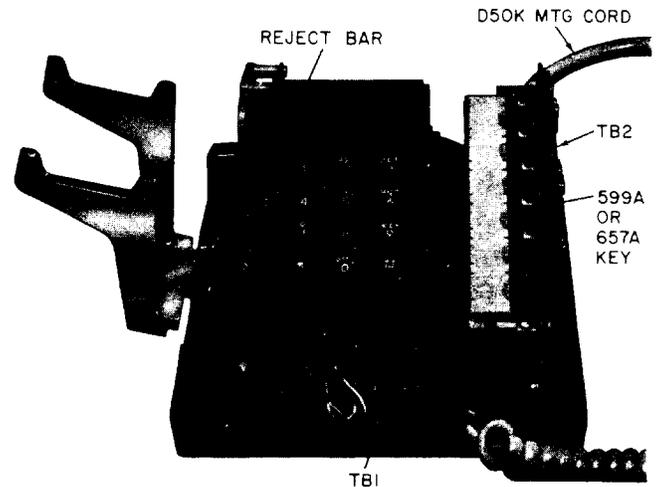
Fig. 2—F-58555 Telephone Set, Interior View
