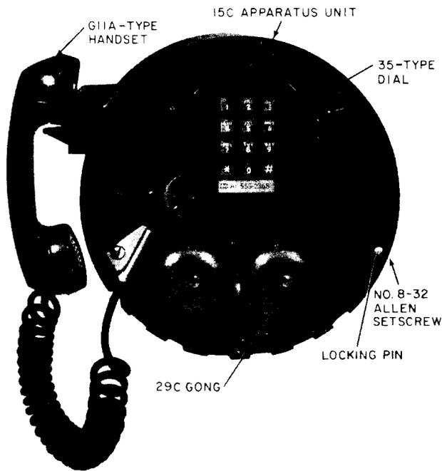
Fig. 2—2520B Telephone Set, Cover Removed
