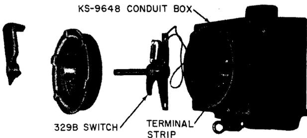
Fig. 4—KS-14547 Foot Switch, Interval View
