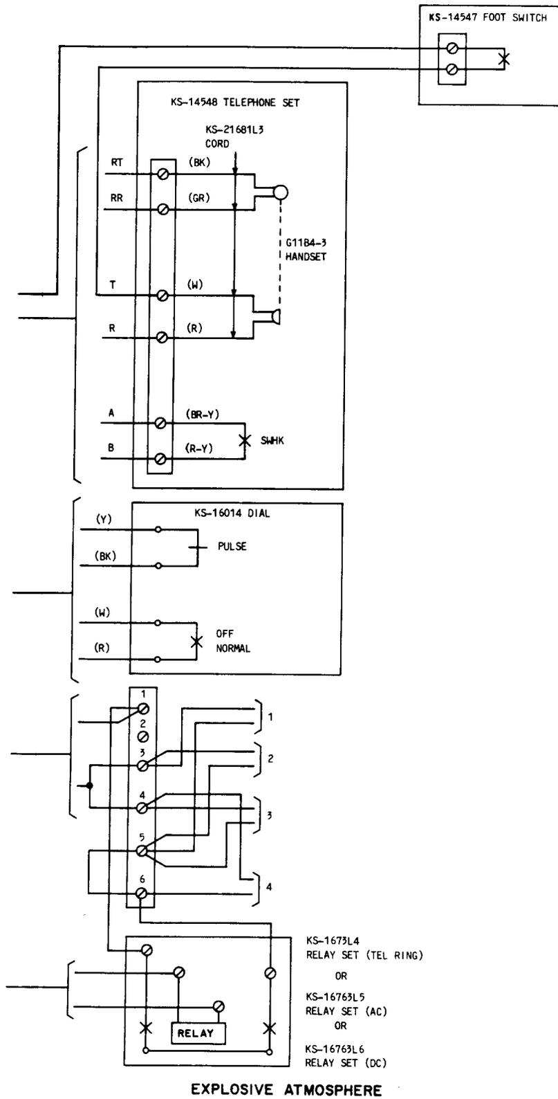
Fig. 8—KS-14548 Telephone Set, Connections (Sheet 2 of 2)
