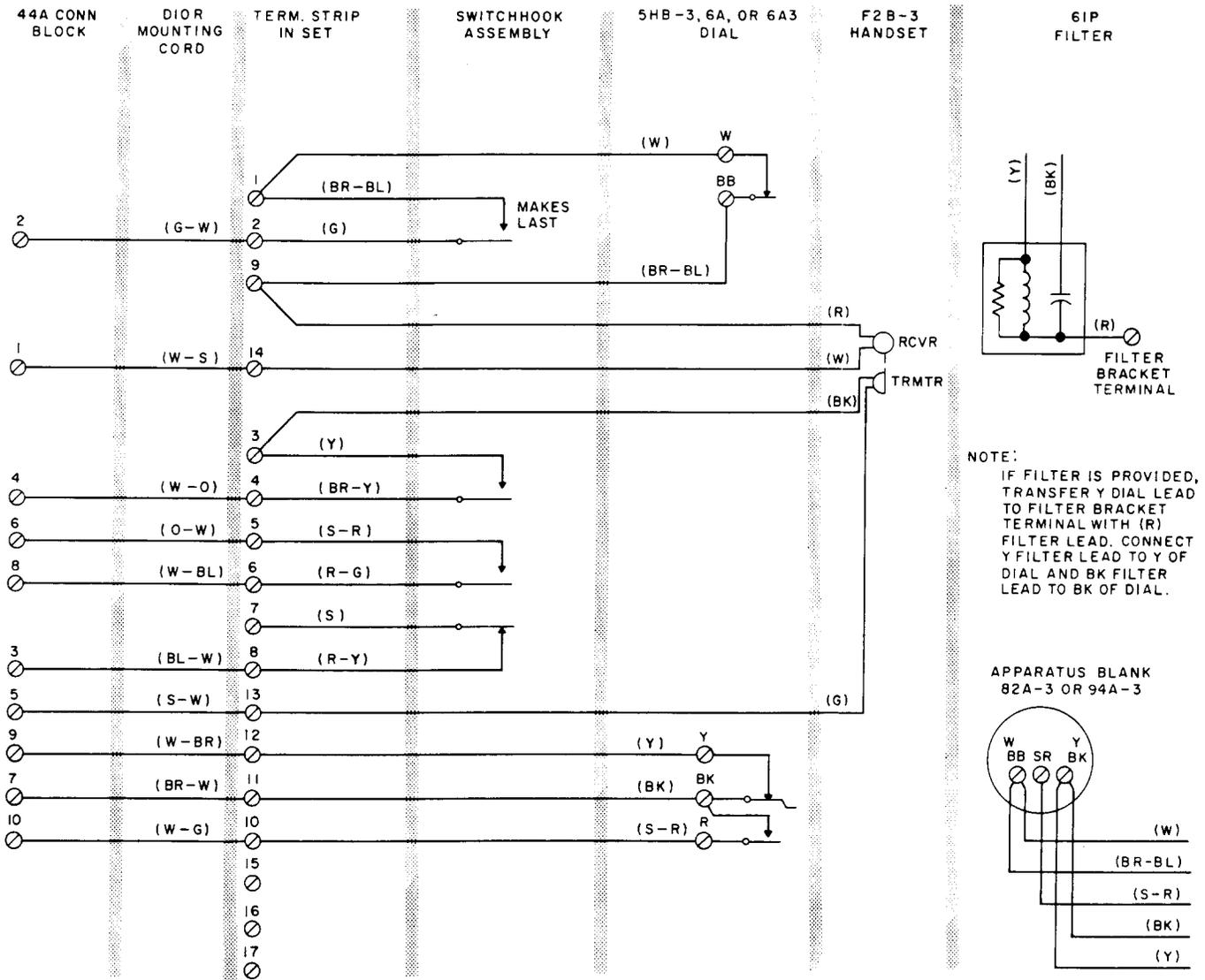
Fig. 2 — 329C Telephone Set — Connections
