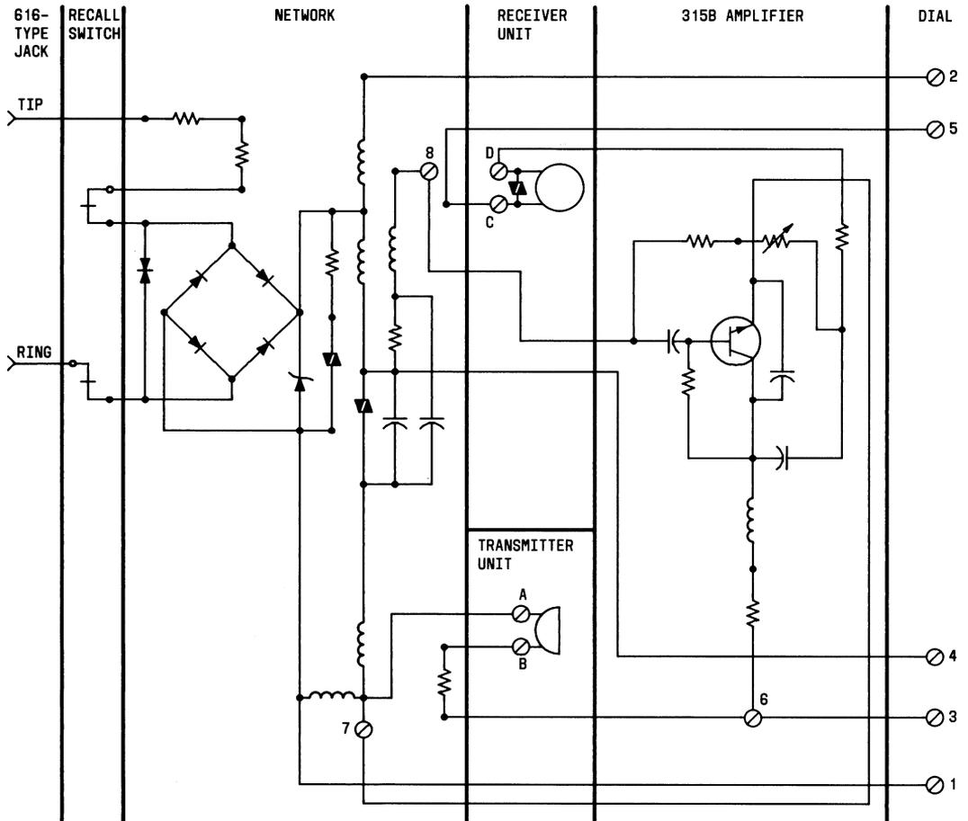
Fig. 31—Schematic of 2226A Hand Telephone Set
