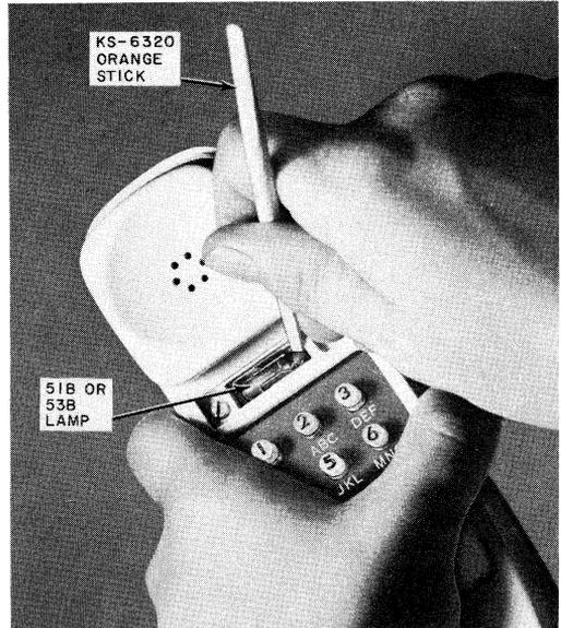
Fig. 18—Removing Dial Lamp From 2220BM Hand Telephone Set
