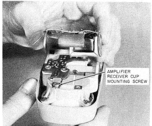
**Fig. 21—Fastening Amplifier to Receiver Unit Cup of Hand Telephone Set**
