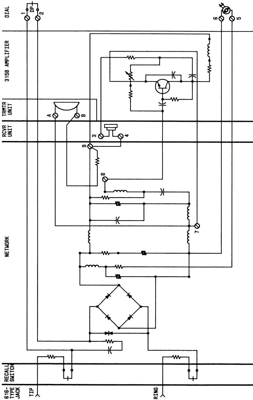
Fig. 28—Schematic of 226A Hand Telephone Set With 315B Amplifier
