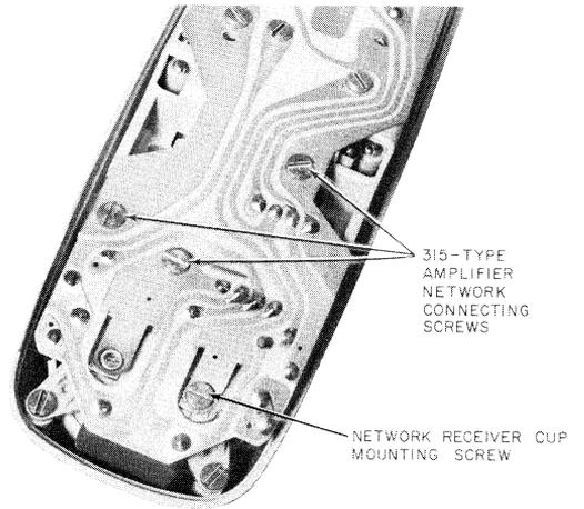
**Fig. 20—Location of Mounting Screws Used to Connect Amplifier in Hand Telephone Set**
