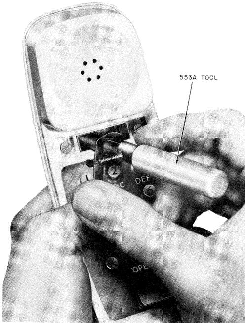
**Fig. 19—Removing Dial Lamp Using 553A Tool**
