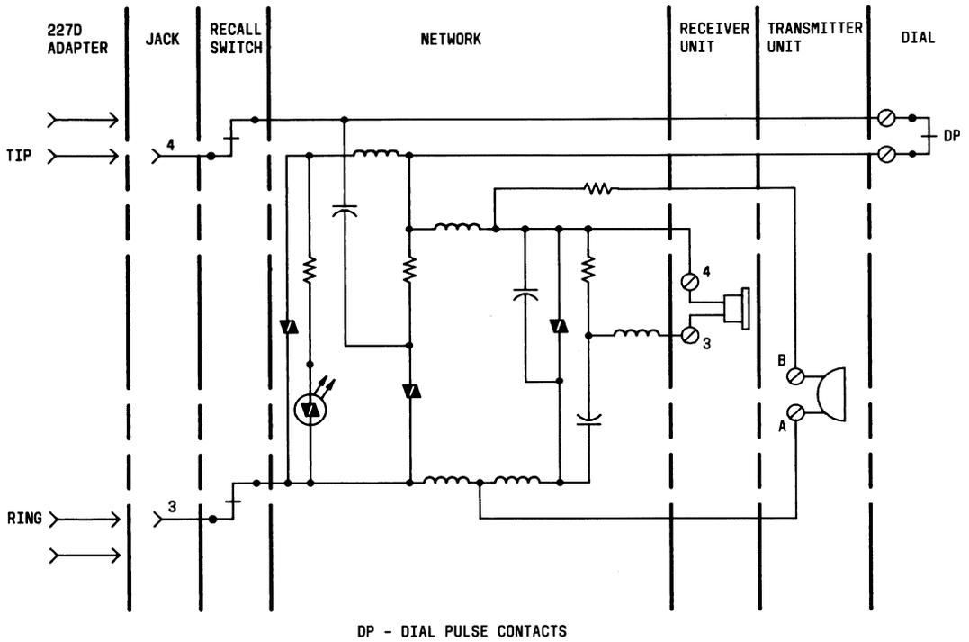
Fig. 26—Schematic of 220AL Hand Telephone Set
