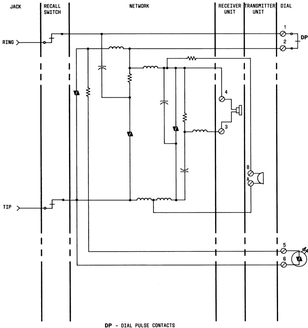
Fig. 25—Schematic of 220C Hand Telephone Set
