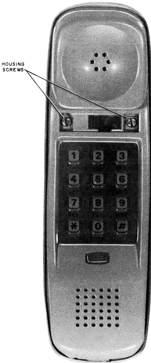
**Fig. 6—Location of Housing Screws**
