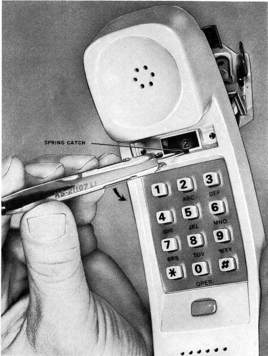
Fig. 22—Releasing Spring Catch on 315-Type Amplifier
