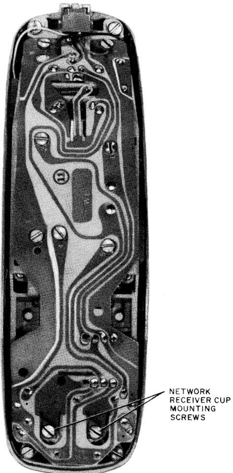
**Fig. 15—2220C Hand Telephone Set Showing Location of Network Mounting Screws**
