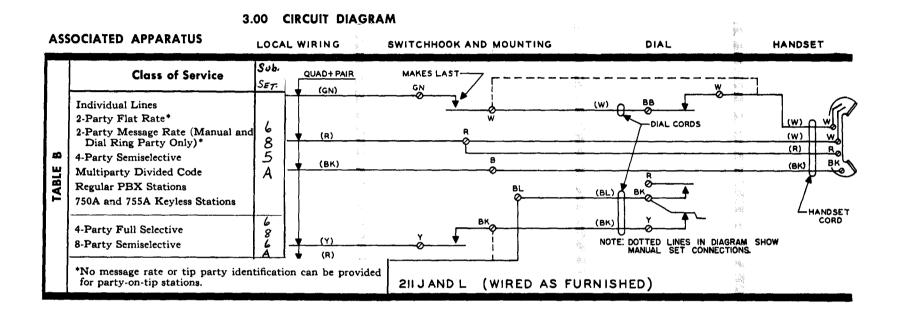
3.01 The 211-type set is arranged for, but not equipped with, a 61M filter for radio-frequency suppression. When this filter is required, remove the dial cord between Y of the dial and BK of the switchhook and connect filter as shown in Fig. 7.
