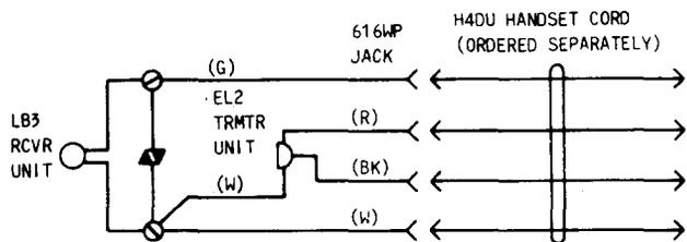
Fig. 2—M1A Handset, Internal Connection
