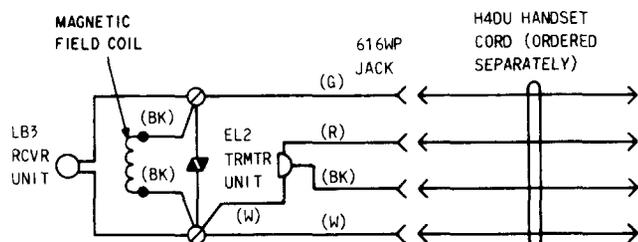
Fig. 3—M2A Handset, Internal Connection
