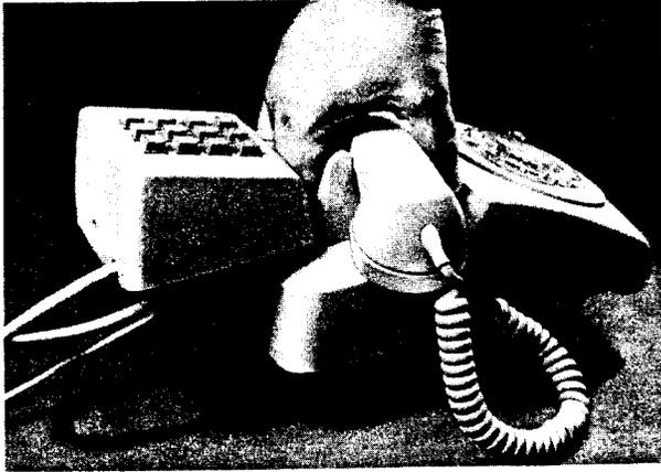
Fig. 5—1035C3A (MD) or 1035AF3A Dial Mounted on 500-Type Telephone Set Using 109B Bracket
