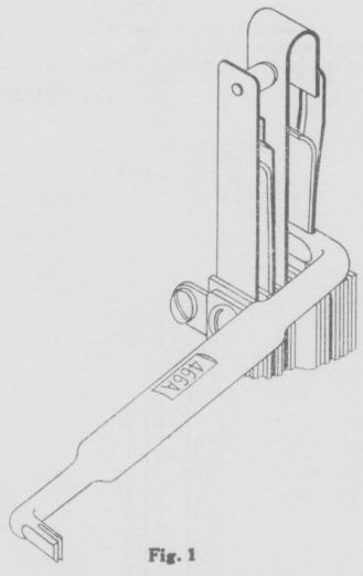
Contact Follow: All contacts shall have a perceptible follow (approximately 1/64") and pairs of contacts of twin contacts shall make at approximately same time. Adjust short contact springs if necessary. In case of springs having stop springs, bend both springs simultaneously when adjusting for follow, but bend only spring finger when adjusting for making at same time.
