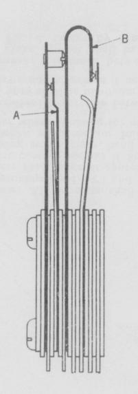
Min. 1/32" Clearance between Springs A and B
