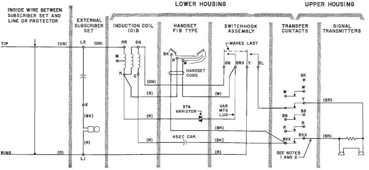
Note 1: If the BR lead does not reach the BKX terminal in upper housing, it is terminated on the A or E terminal on coin chute. A red-white strap connects A or E and BKX.
