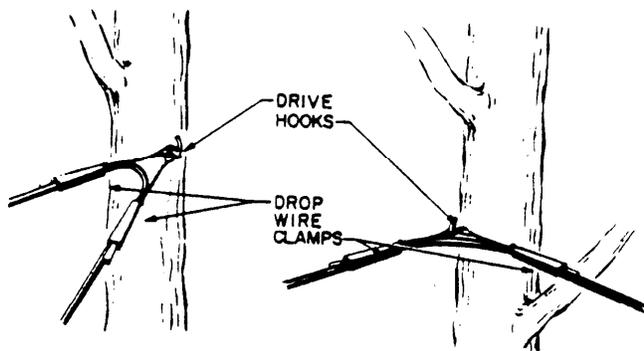
Fig. 16-Turning Corner on Large Diameter Trees
