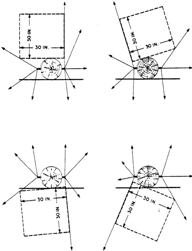
Fig. 1-Drop Wires Distributed from Pole
