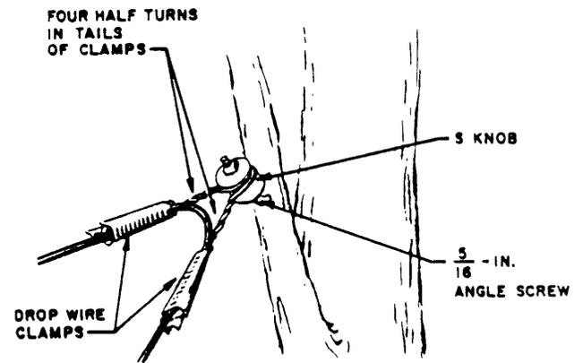
Fig. 18—Turning Corner on Small Diameter Tree
