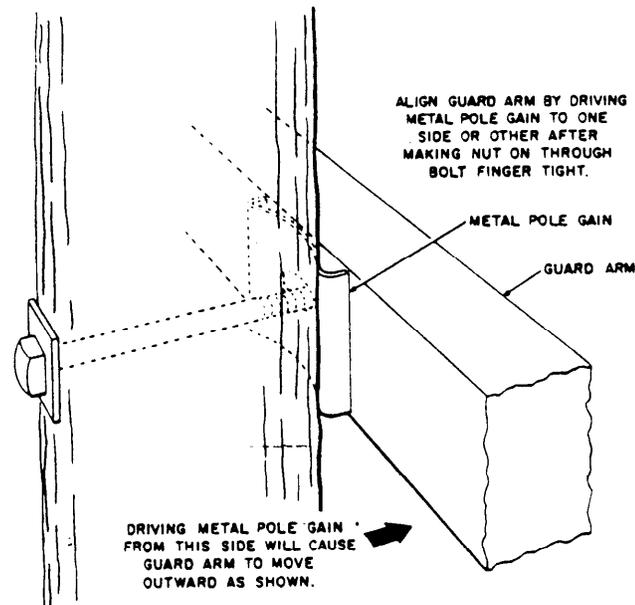
Fig. 6-Metal Pole Gain Installed
