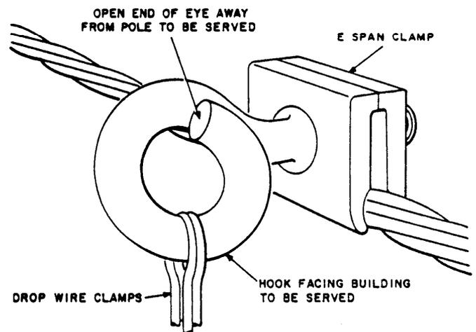
Fig. 22-E Span Clamp Mounted on Strand
