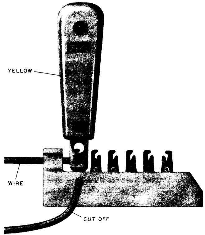
Fig. 10—Ended Termination Completed
