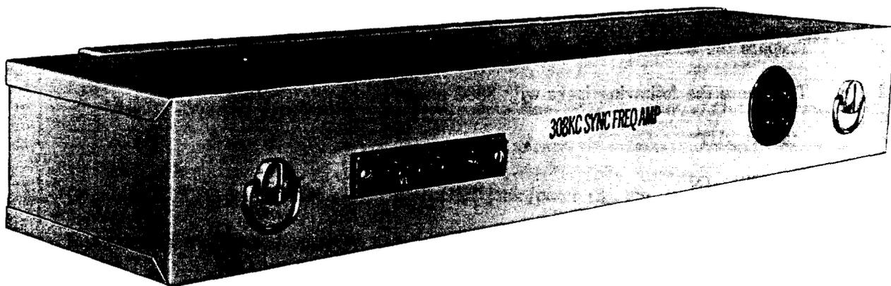
Fig. 1—308-kHz Synchronizing Frequency Converter—Front View
