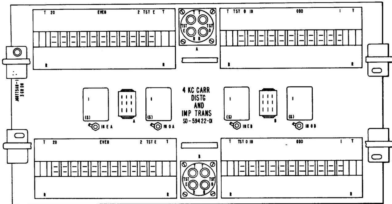
Fig. 1—J68775AU 4-kHz Carrier Distribution and Impedance Transformation Unit (Front Cover Removed)
