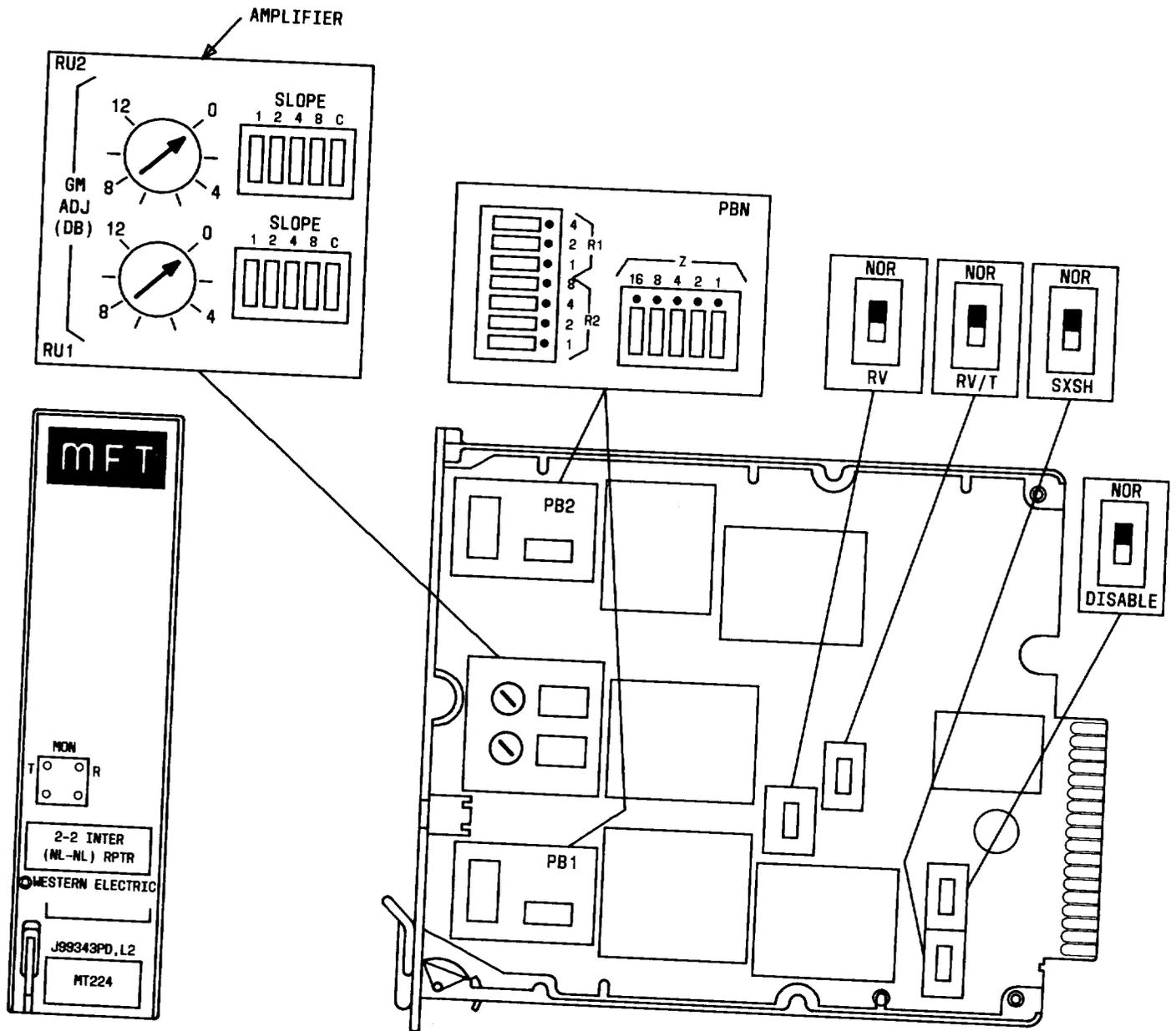
Fig. 2—2-2 Intermediate (NL-NL) Repeater J99343PD, L2 (MD) Component Layout
