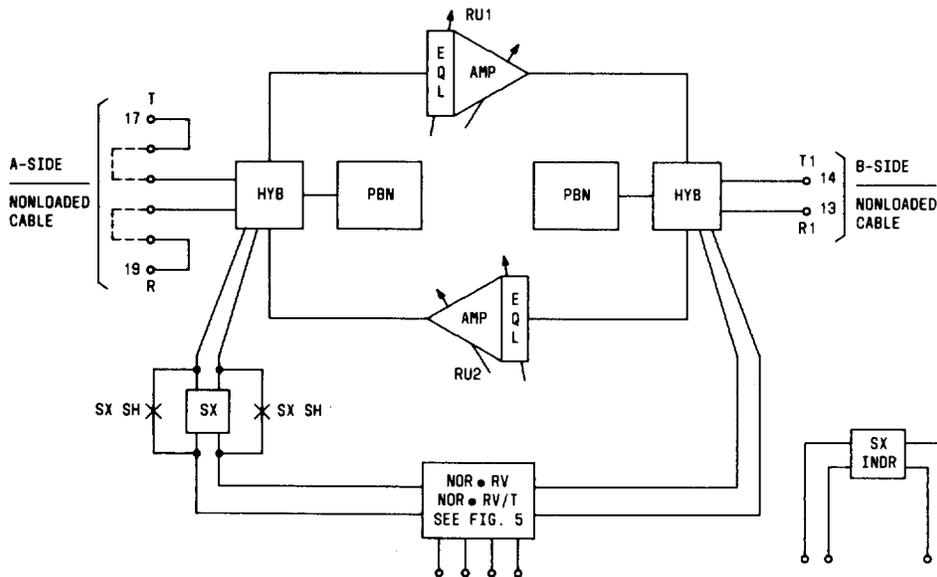
Fig. 3—Block Diagram of the 2-2 Intermediate (NL-NL) Repeater J99343PD, L1 and L2
