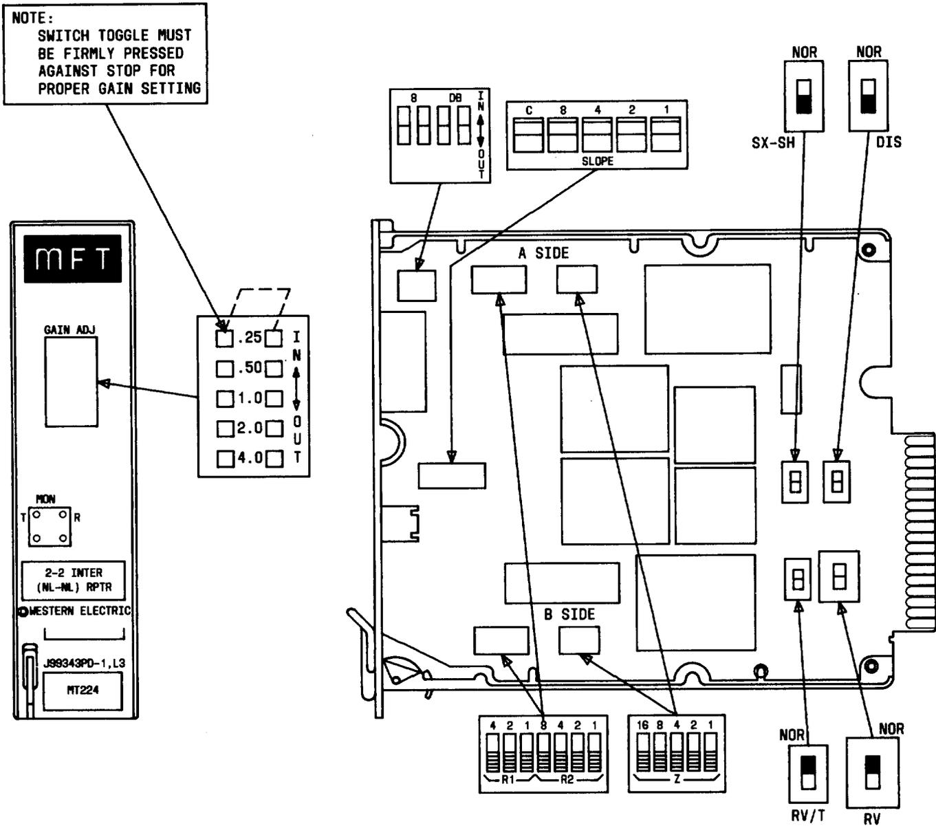
Fig. 6—2-2 Intermediate (NL-NL) Repeater J99343PD, L3 Component Layout
