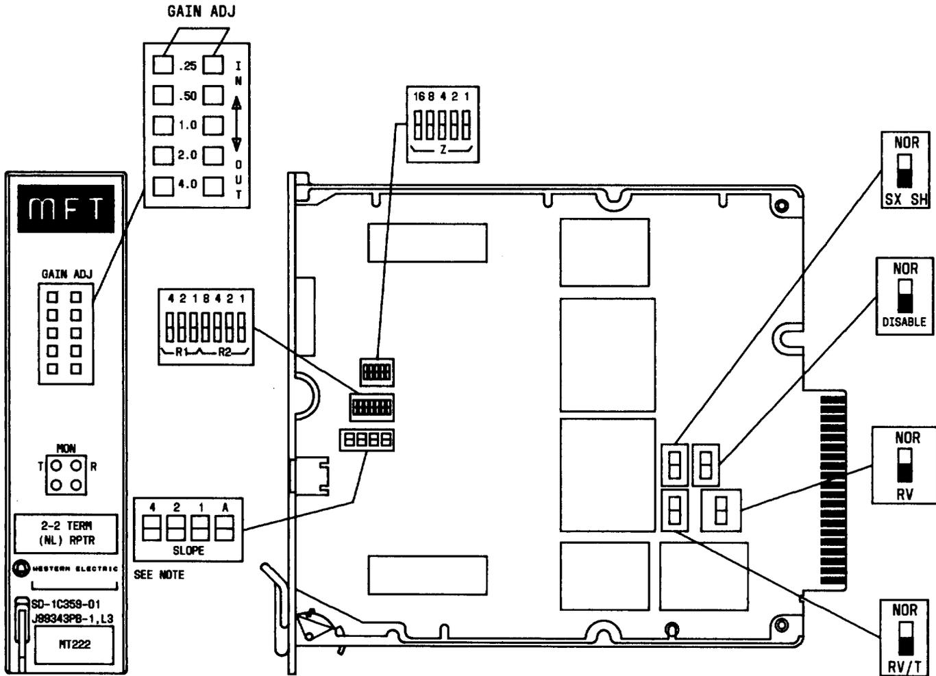
NOTE: THE "A" SWITCH DOES NOT PERFORM THE SAME FUNCTION AS THE "C" SWITCH ON J99343PB-1, L1 & L2.
