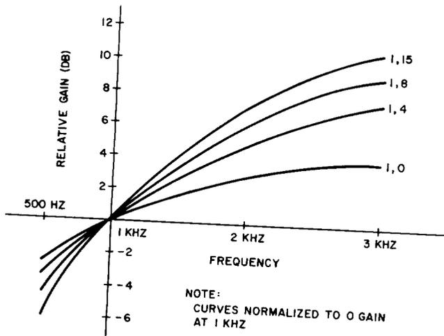
Fig. 9—Amplifier/Equalizer Response C=1
