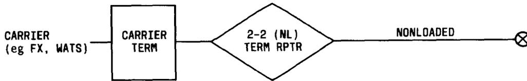
2-WIRE (NL) EXTENSION OFF CARRIER OR FX TRUNK
