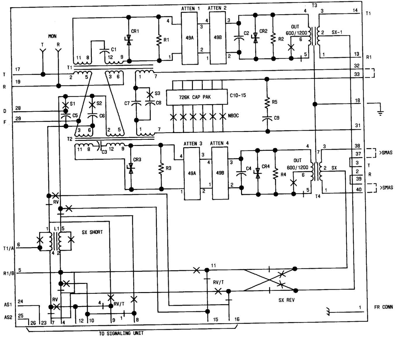
Fig. 3—J99343BE 2-4 Wire Transmission Unit—Schematic Diagram
