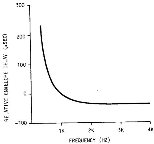
**Fig. 7—2-4 Wire Transmission Unit Relative Envelope Delay**
