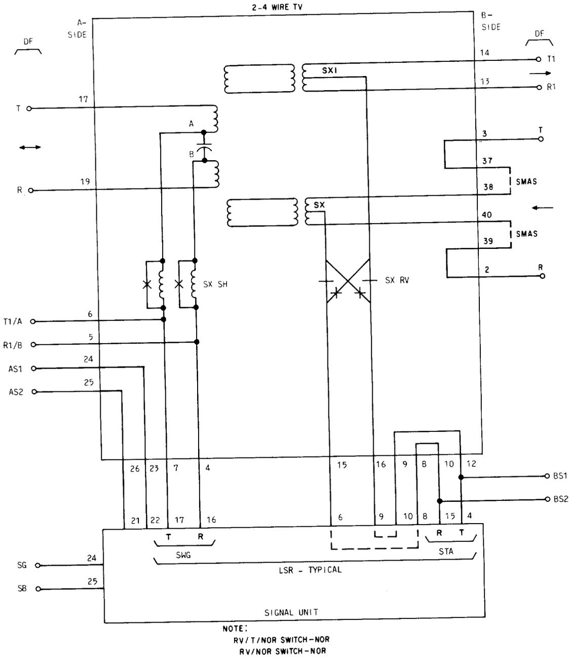
Fig. 4—2-4 Wire Transmission Unit Signaling Lead Access—Normal Signaling
