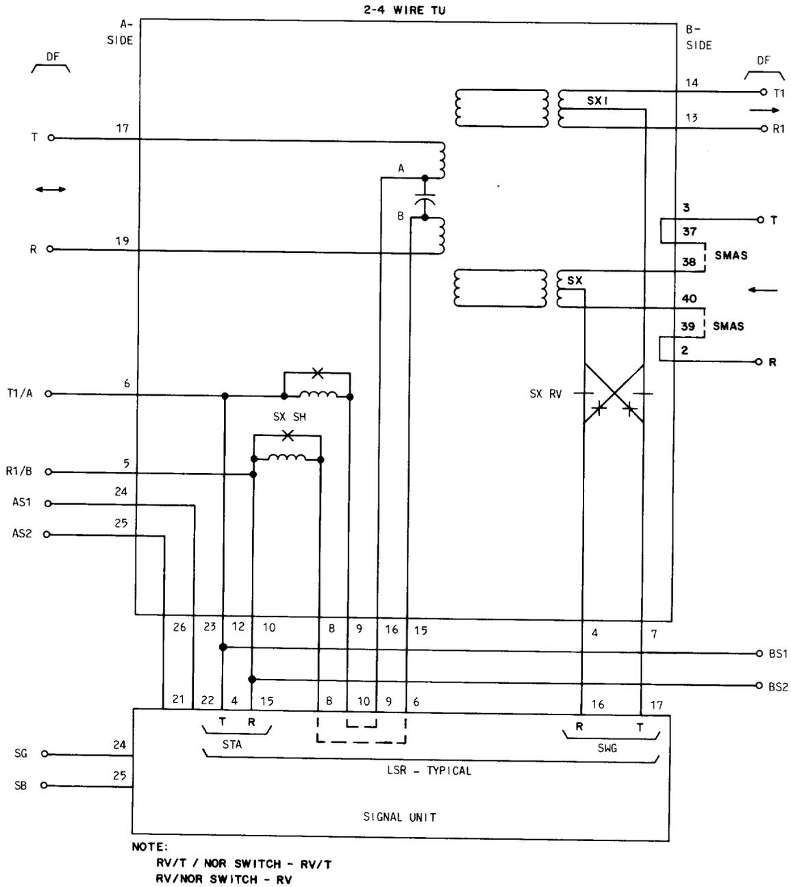
Fig. 5—2-4 Wire Transmission Unit Signaling Lead Access—Reverse Signaling
