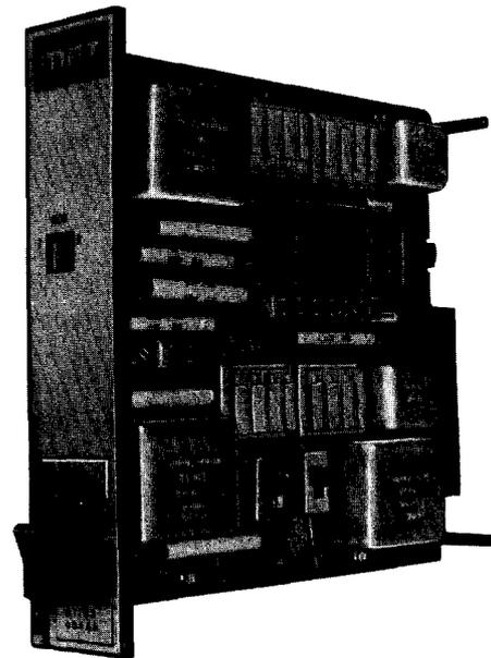
Fig. 1—2-4 Wire Transmission Unit
