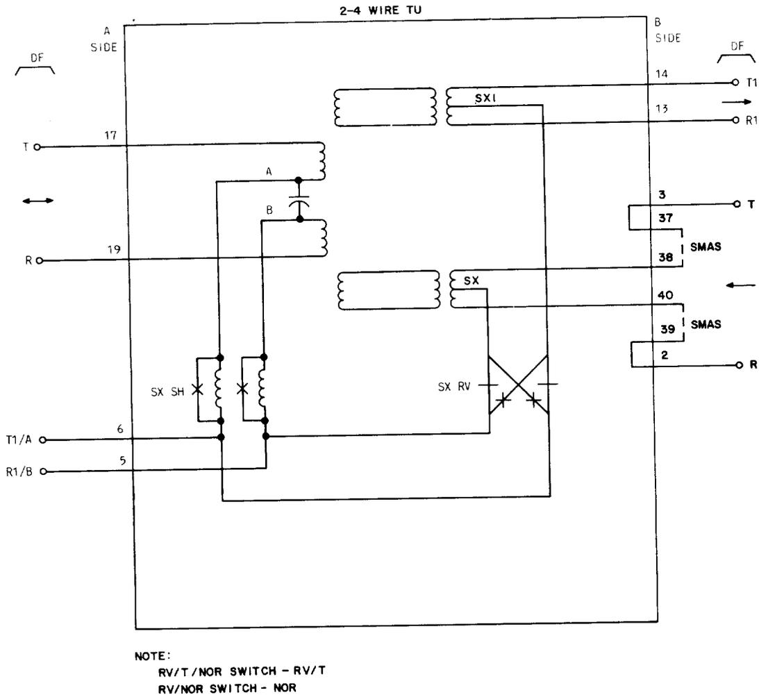
**Fig. 6—2-4 Wire Transmission Unit Signaling Lead Access—Through Signaling**
