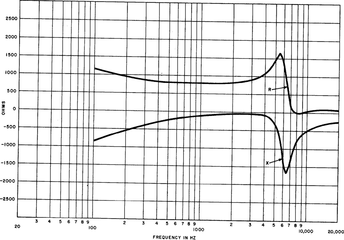
Fig. 3 — 4066E Network — Midsection Impedance — Simulating 19H44-S Cable
