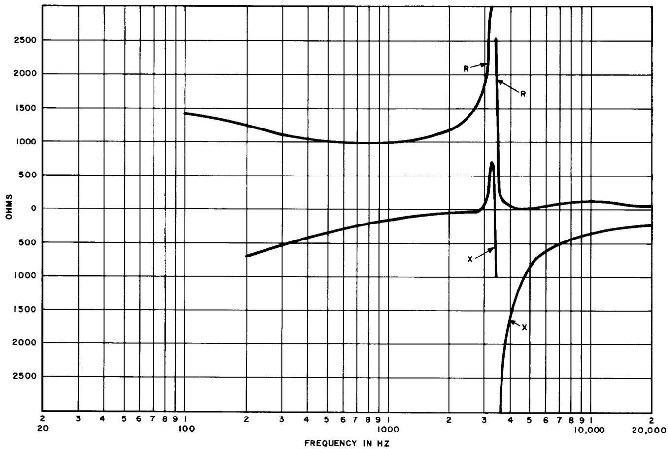
Fig. 11—4066A Network—Simulating Midsection Impedance of 22H88 High-Capacitance Cable
