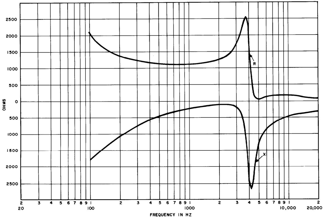
Fig. 13—4066A Network—Simulating Midsection Impedance of 24H88 Low-Capacitance Cable
