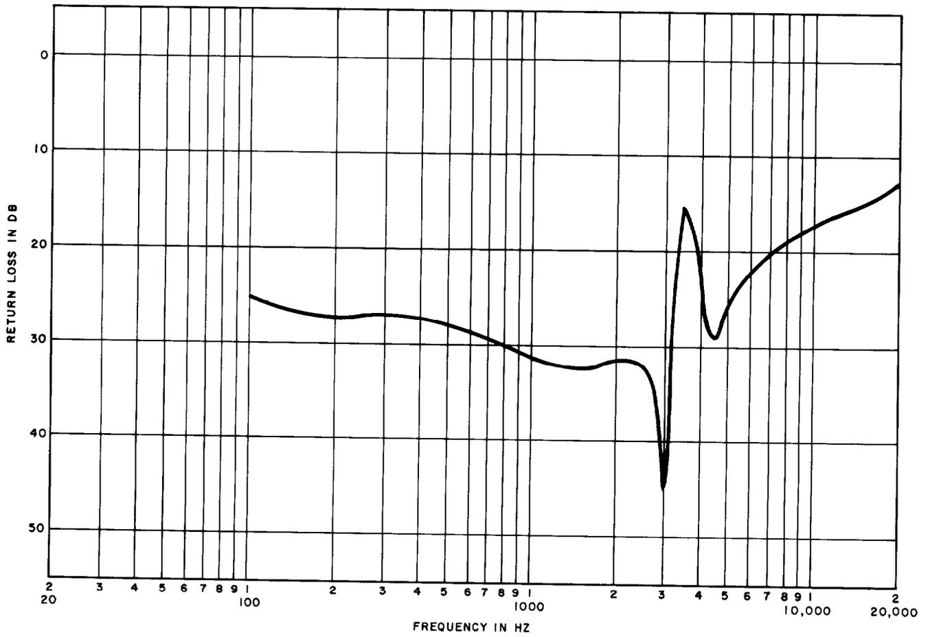
Fig. 5—4066A Network—Return Loss vs 24H88 High-Capacitance Cable—End Section = 0.5 Loading Section
