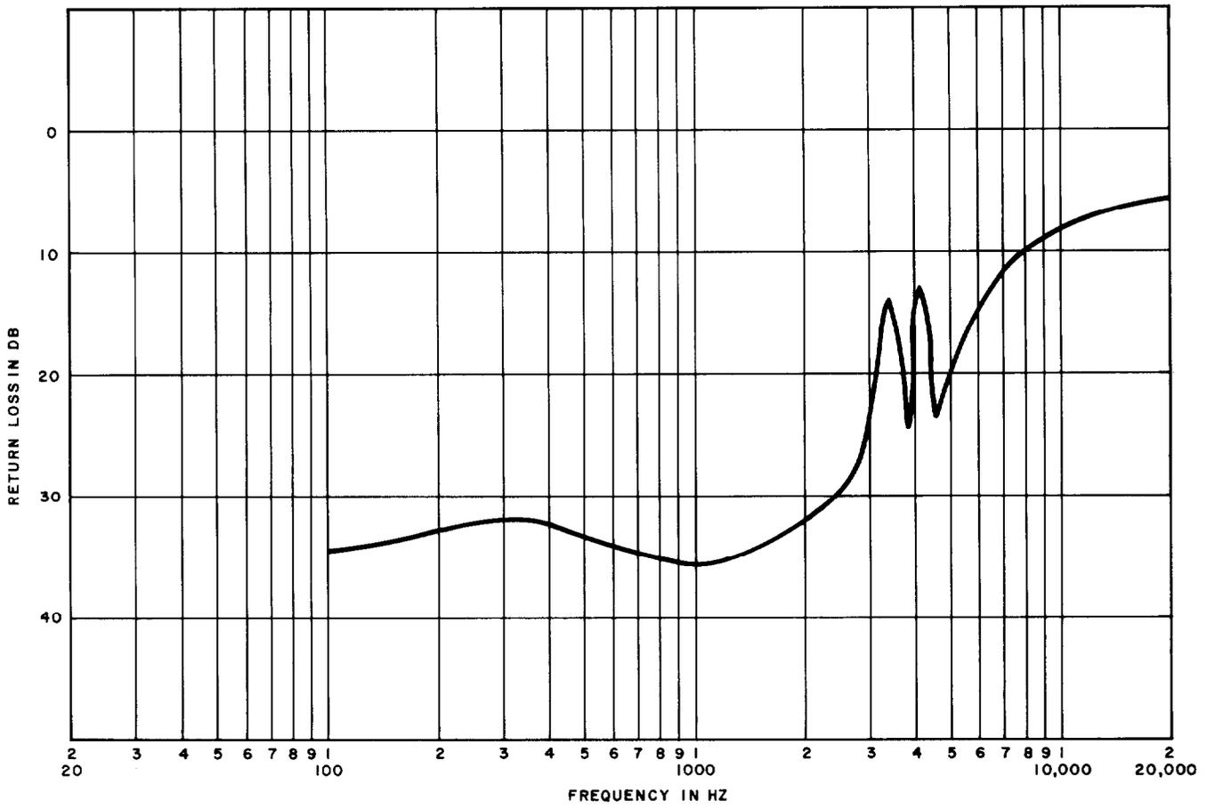
Fig. 8—4066A Network—Return Loss vs 19H88 High-Capacitance Cable—End Section = 0.25 Loading Section
