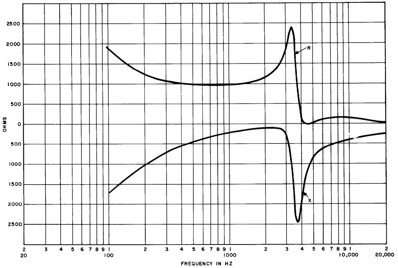
Fig. 12—4066A Network—Simulating Midsection Impedance of 24H88 High-Capacitance Cable
