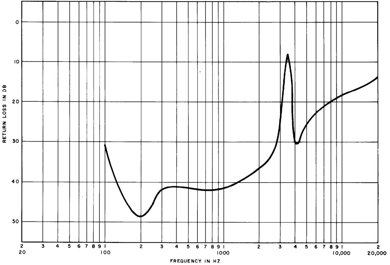
Fig. 4—4066A Network—Return Loss vs 22H88 High-Capacitance Cable—End Section = 0.5 Loading Section
