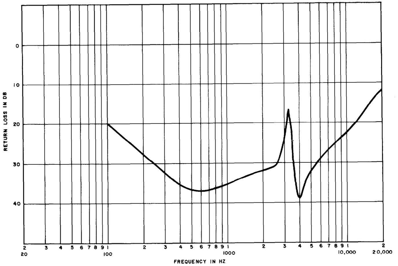
Fig. 7—4066A Network—Return Loss vs 19H88 High-Capacitance Cable—End Section = 0.75 Loading Section
