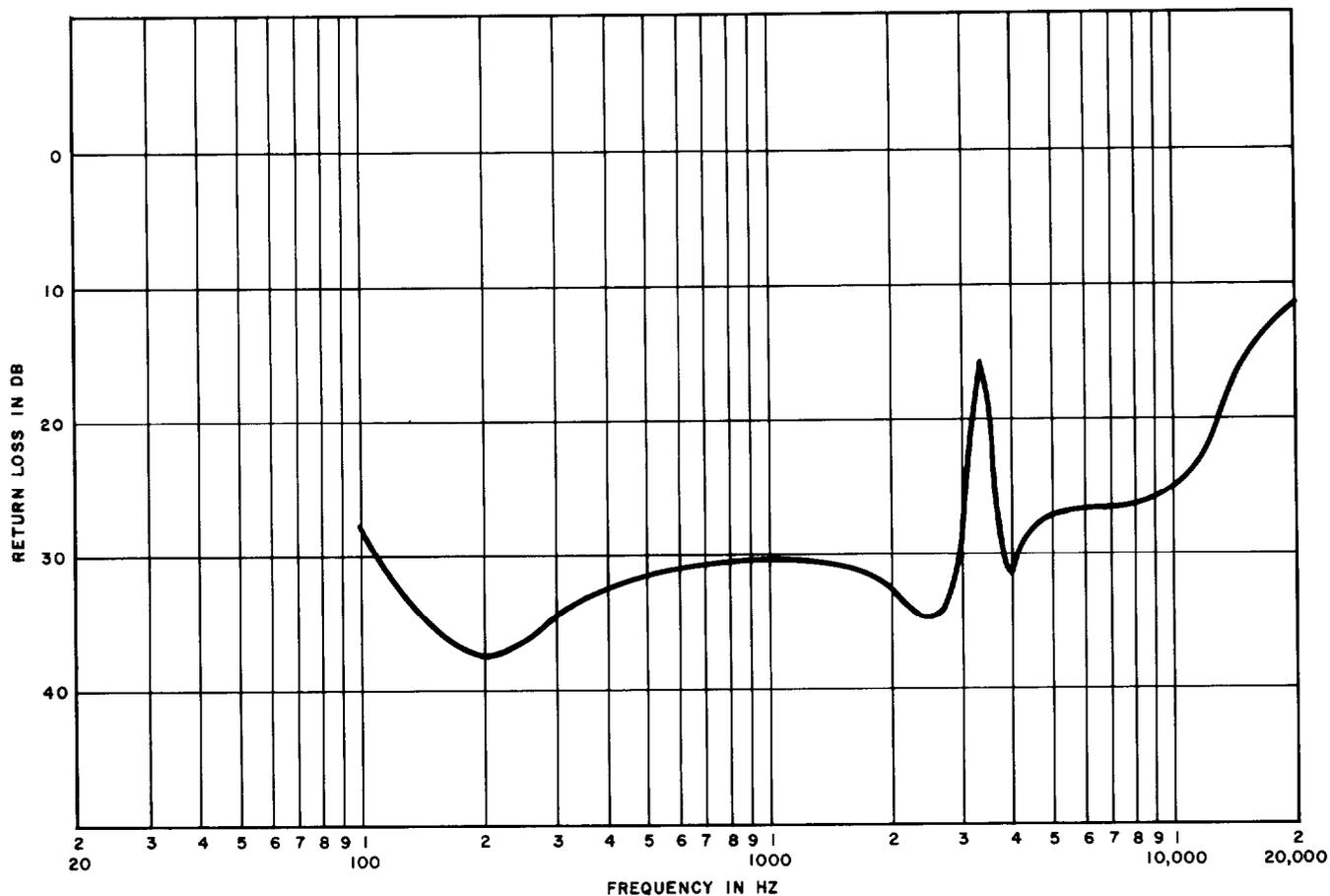
Fig. 9—4066A Network—Return Loss vs 22H88 High-Capacitance Cable—End Section = 0.75 Loading Section
