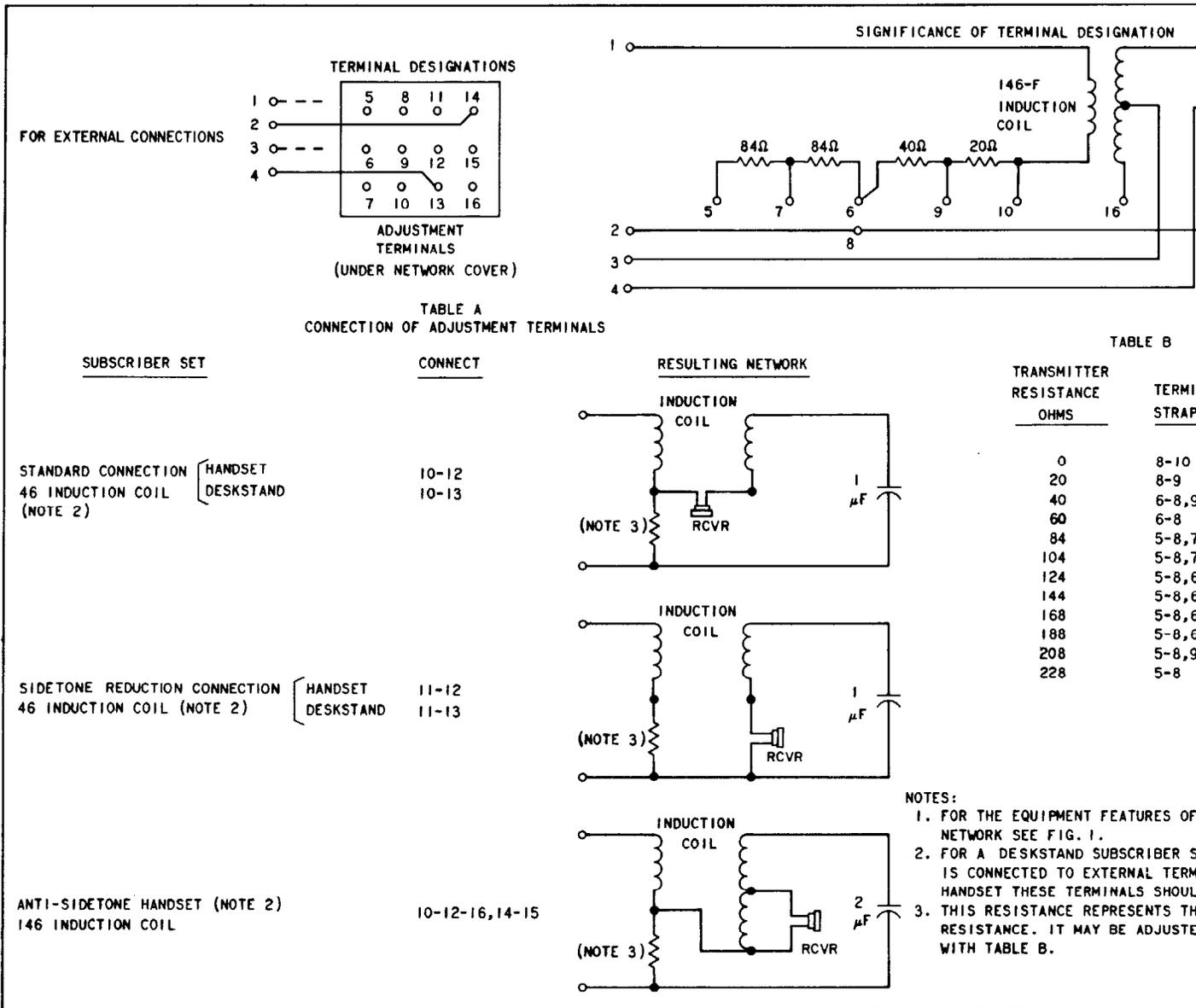
**Fig. 4—113F Balancing Network for Subscriber Sets**
