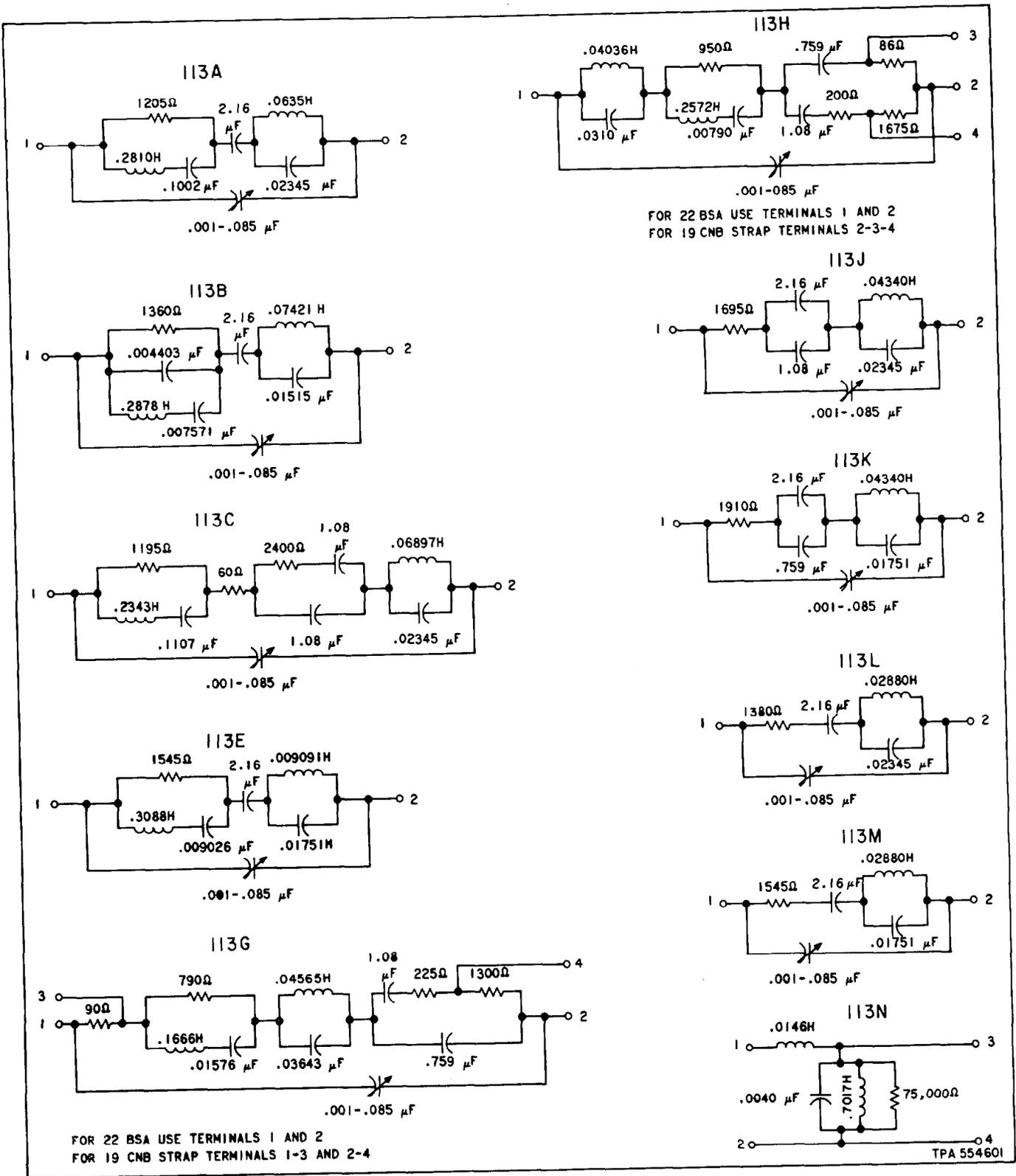
Fig. 2—113-Type Networks for Exchange Facilities
