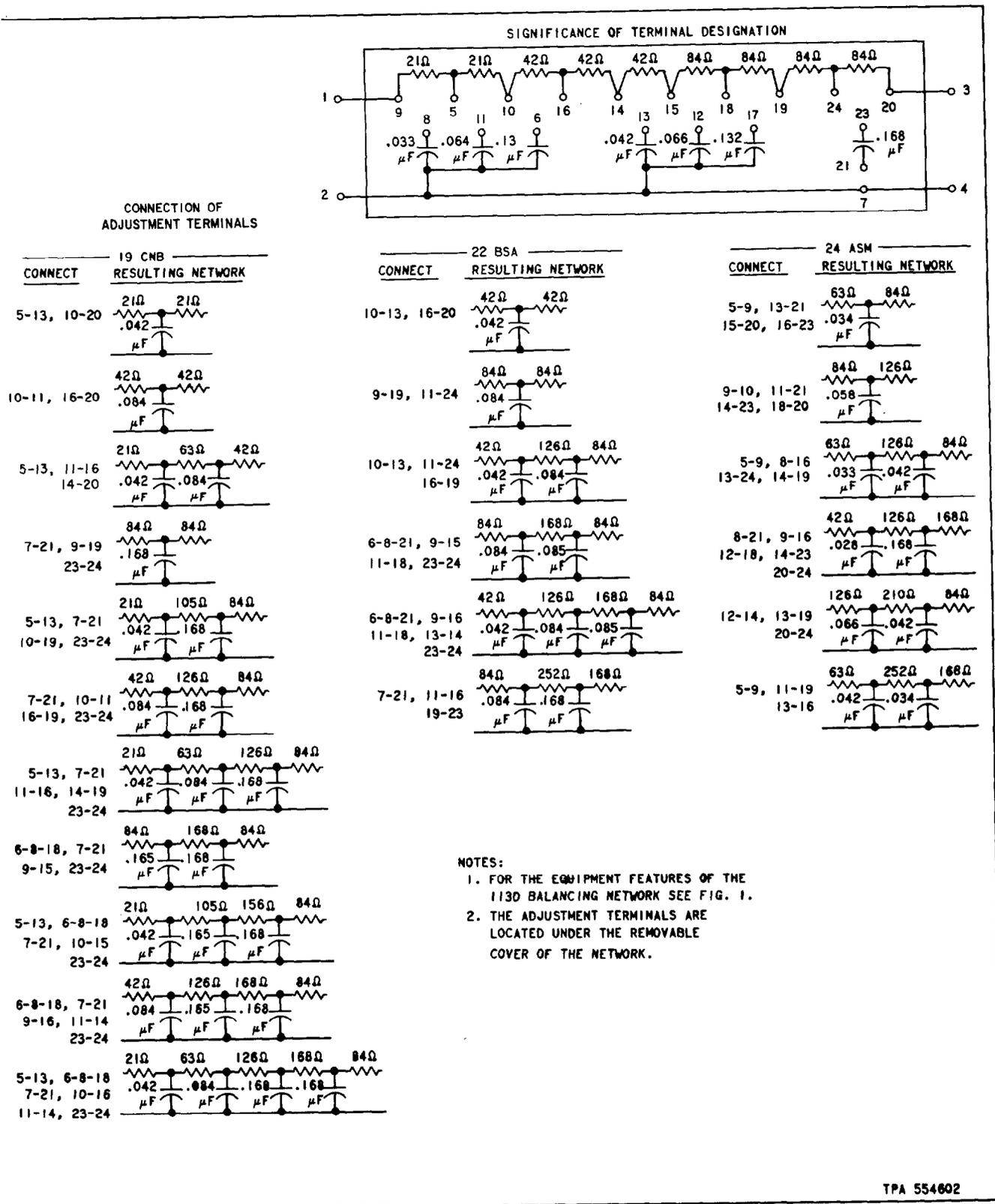
Fig. 3—113D Balancing Network for Nonloaded Cable Circuits
