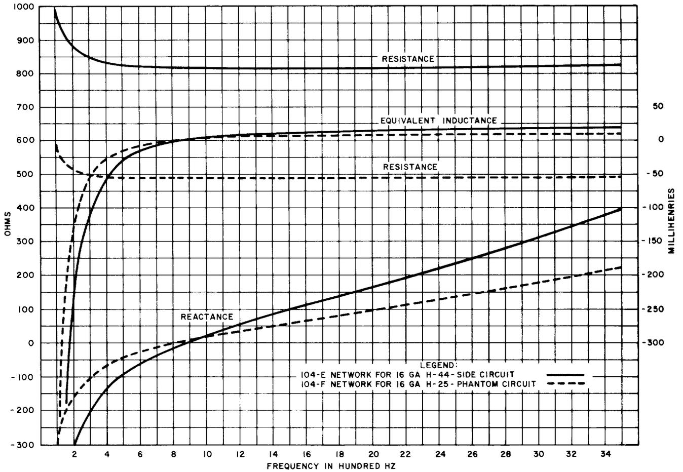
Fig. 10—Impedance of Networks for Toll Cable—104-Type Networks for H-44-25 Circuits
