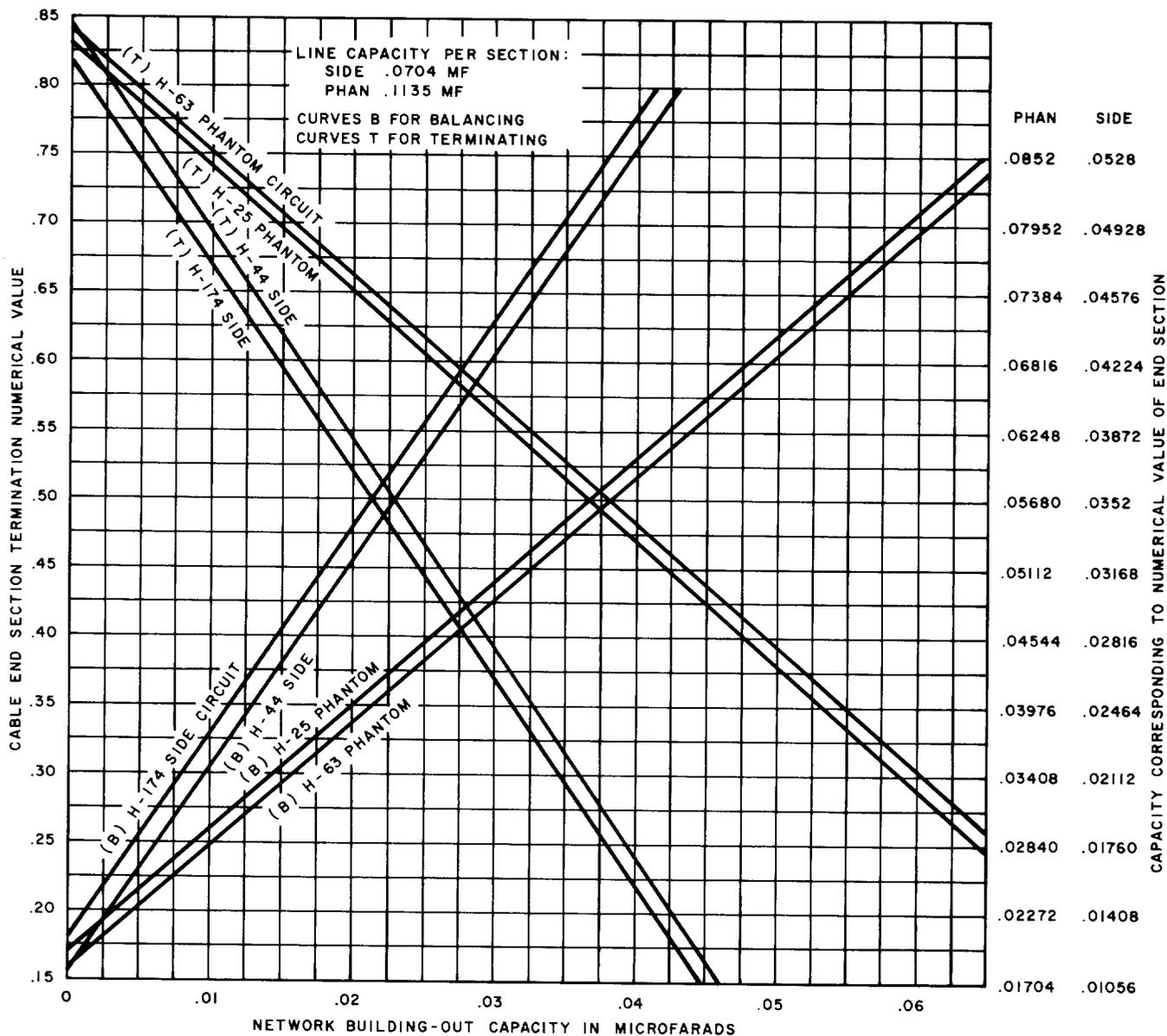
Fig. 20—Network Building-Out Capacity versus Cable End-Section for 104-Type Networks
