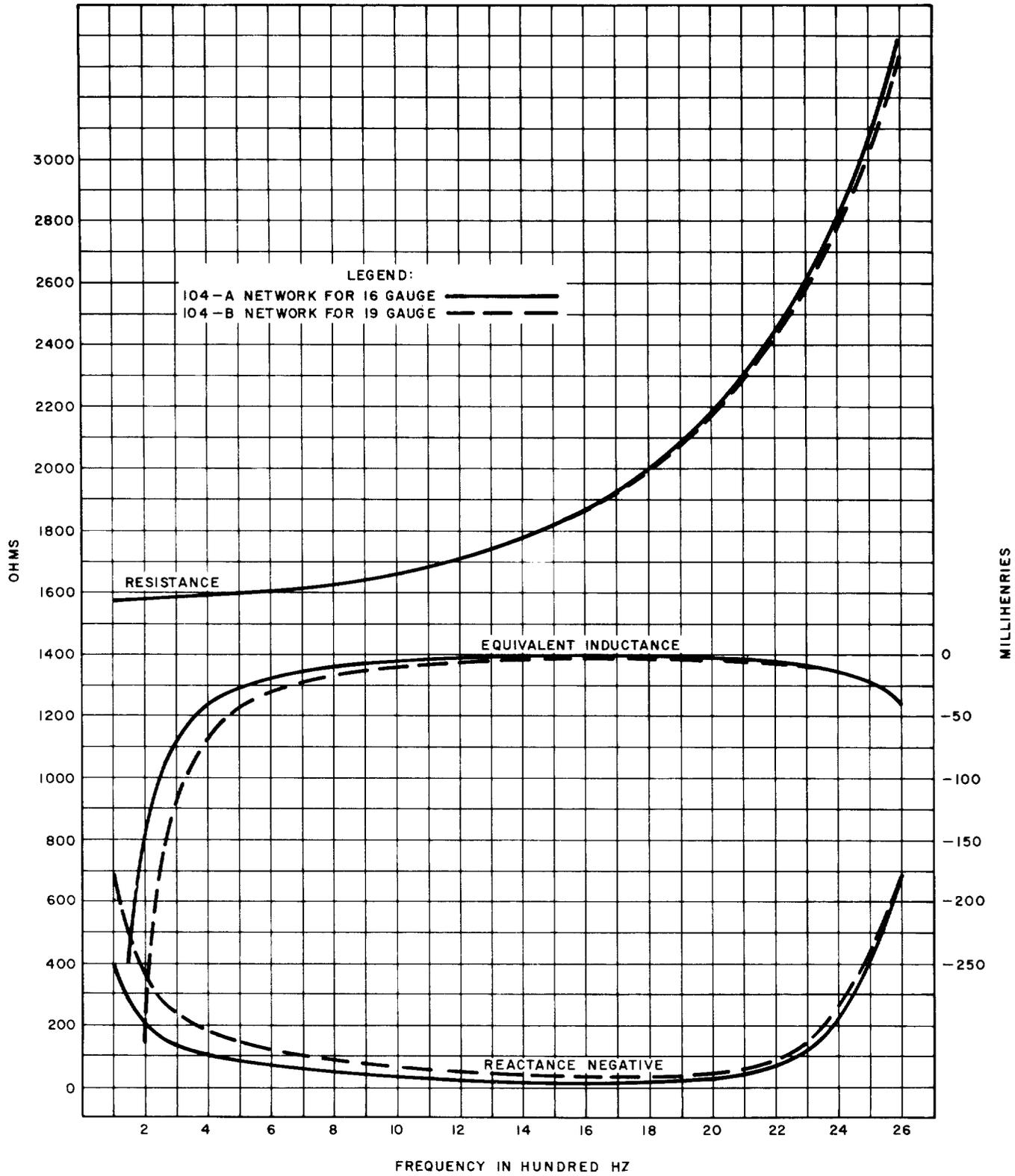
Fig. 5—Mid-Section Impedance of Networks for H172-174 Side Circuits
