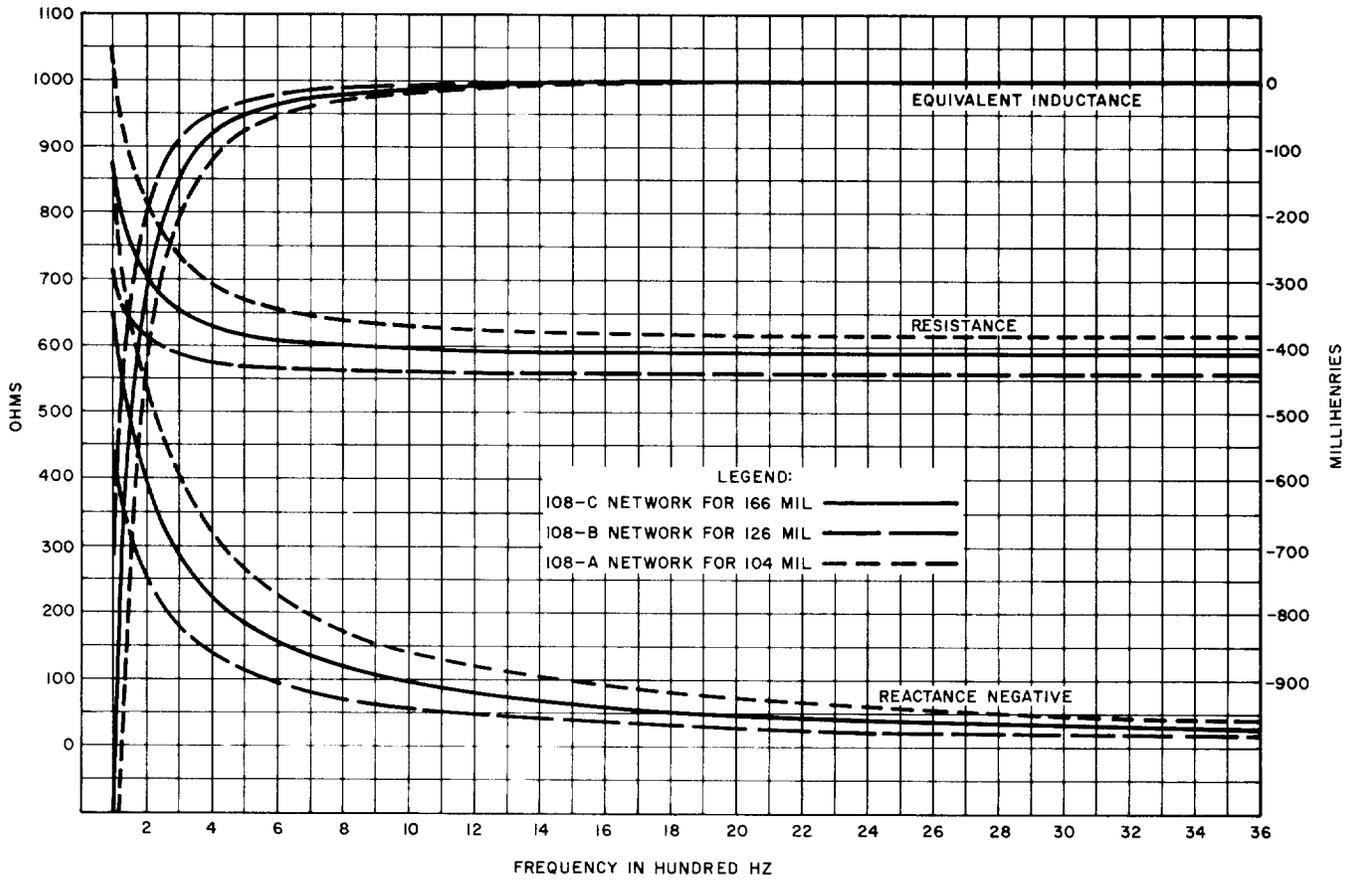
Fig. 19—Impedance of Networks for Toll Entrance Cable—108-Type Networks for H-31-18 Loaded Phantom Circuits
