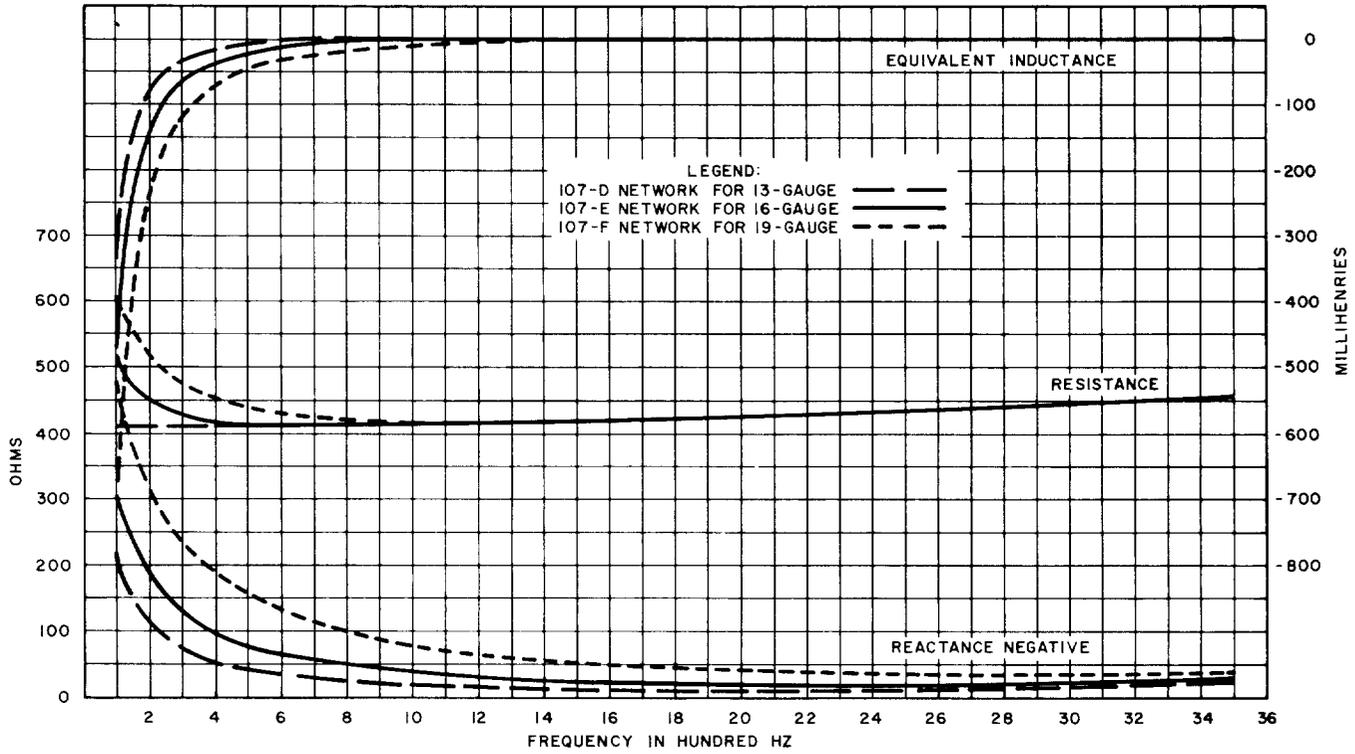
Fig. 17—Mid-Section Impedance of Networks for Toll Entrance Cable—107-Type Networks for H-31-18 Loaded Phantom Circuits
