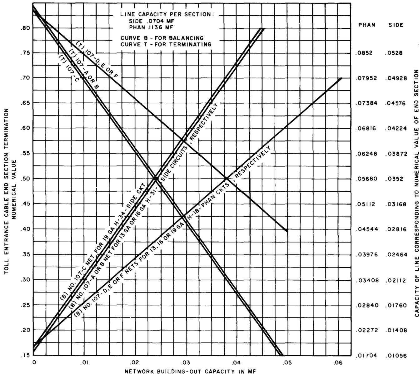
Fig. 22—Network Building-Out Capacity versus Cable End-Section for 107-Type Networks
