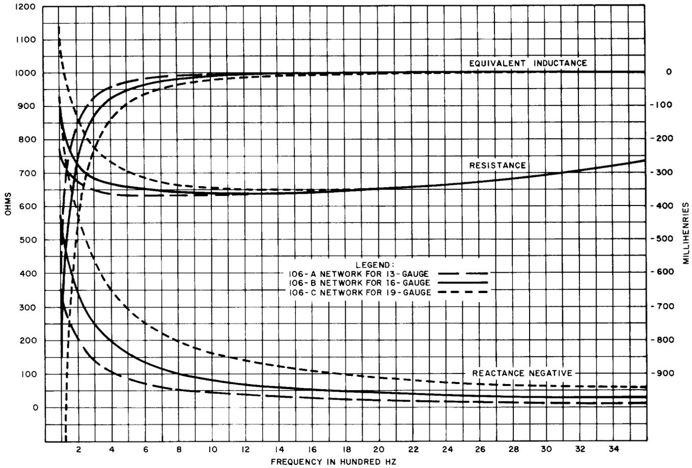
Fig. 11—Mid-Section Impedance of Networks for Toll Entrance Cable—106-Type Networks for H-18-16 Loaded Side Circuits
