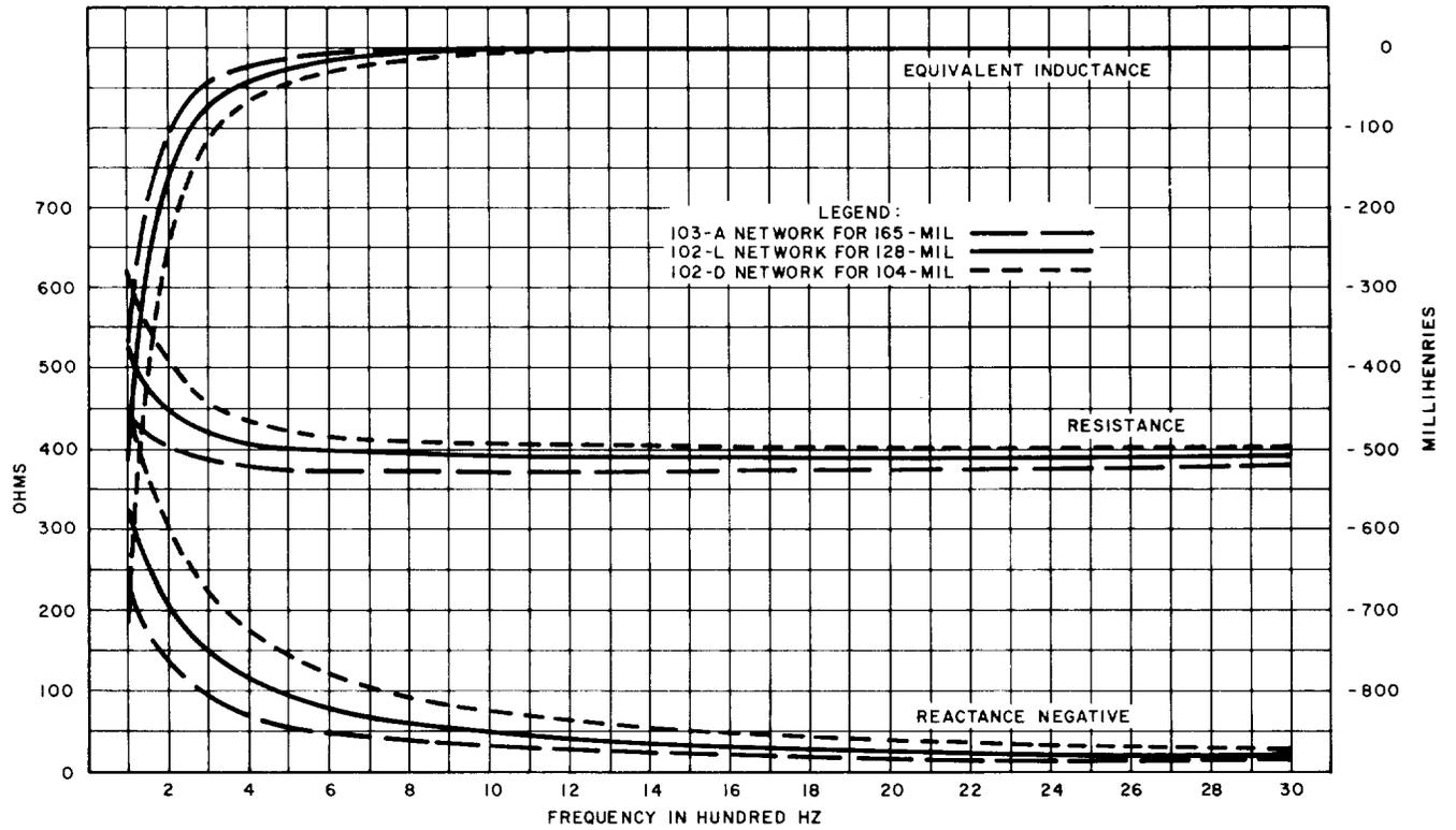
Fig. 4—Impedance of Networks for Nonloaded Open-Wire Circuits—102- and 103-Type Networks for 12-Inch Spaced Phantom Circuits
