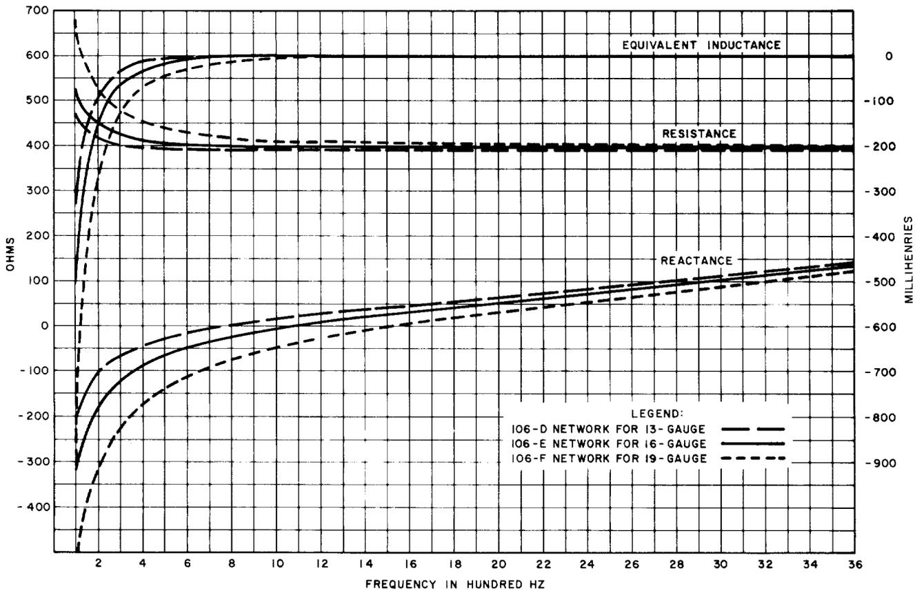
Fig. 14—Impedance of Networks for Toll Entrance Cable—106-Type Networks for H-28-16 Loaded Phantom Circuits
