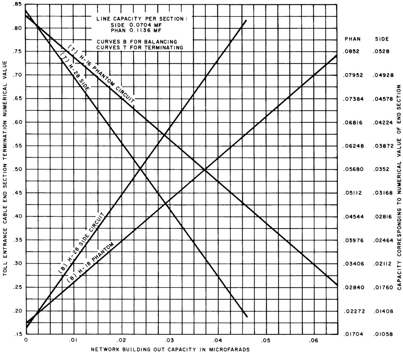
Fig. 21—Network Building-Out Capacity versus Toll Entrance Cable End-Section for H-28-16 Networks
