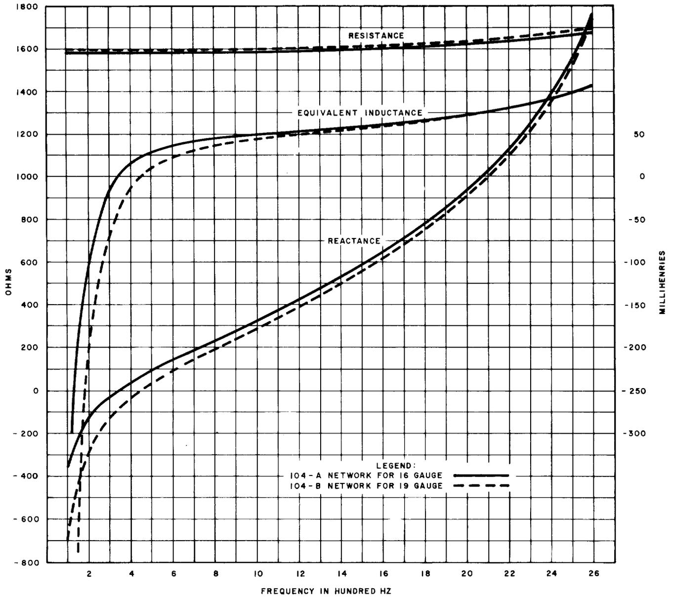
Fig. 6—Impedance of Networks for Nonloaded Open-Wire Circuits—102- and 103-Type Networks for 12-Inch Spaced Phantom Circuits
