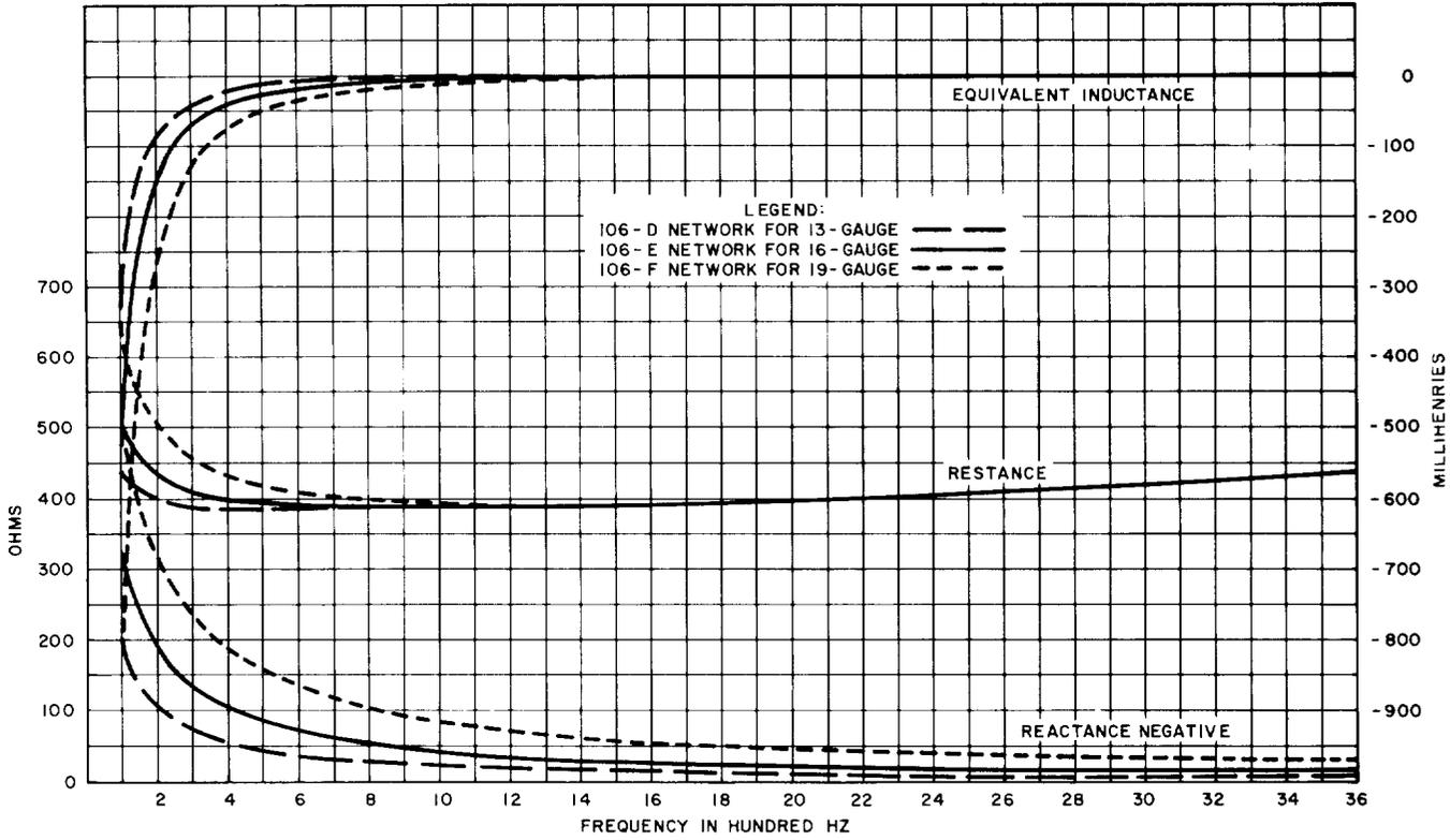
Fig. 13—Mid-Section Impedance of Networks for Toll Entrance Cable—106-Type Networks for H-28-16 Loaded Phantom Circuits
