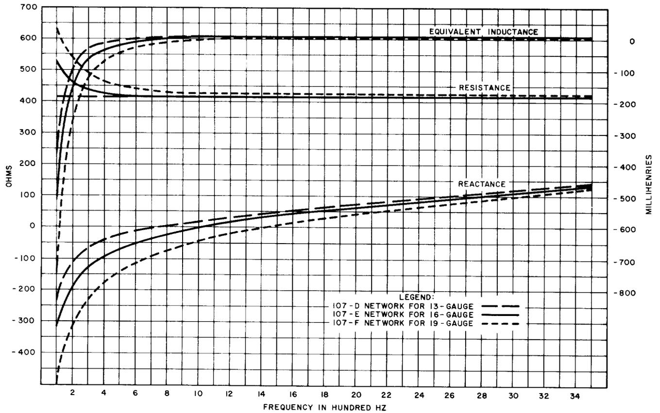
Fig. 18—Impedance of Networks for Toll Entrance Cable—107-Type Networks for H-31-18 Loaded Phantom Circuits
