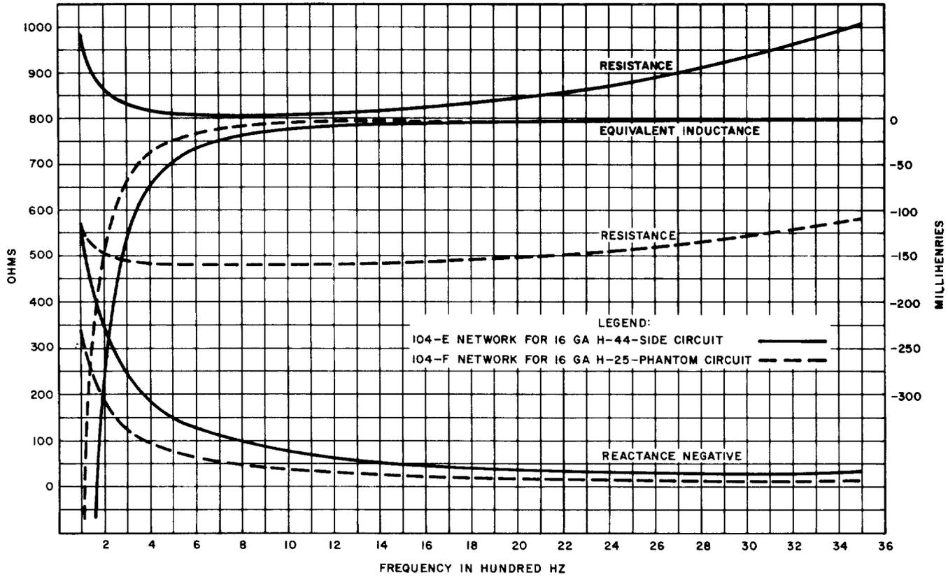
Fig. 9—Mid-Section Impedance of Networks for Toll Cable—104-Type Networks for H-44-25 Circuits
