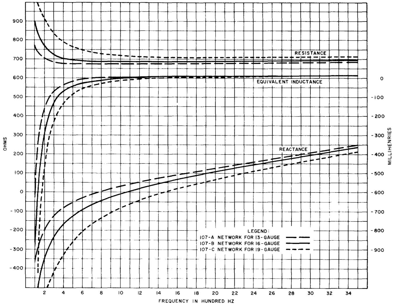
Fig. 16—Impedance of Networks for Toll Entrance Cable—107-Type Networks for H-31-18 Loaded Side Circuits
