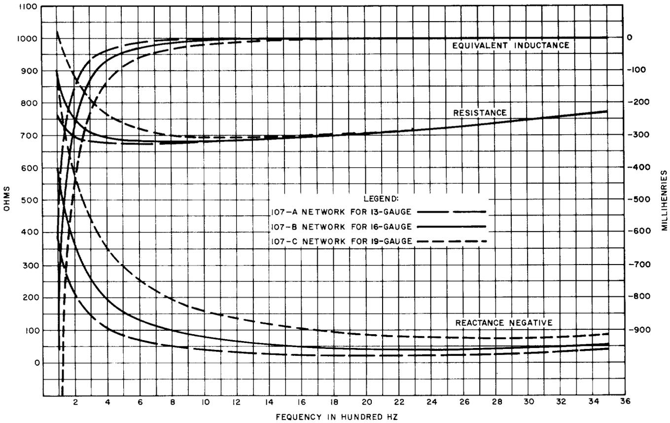
Fig. 15—Mid-Section Impedance of Networks for Toll Entrance Cable—107-Type Networks for H-31-18 Loaded Side Circuits
