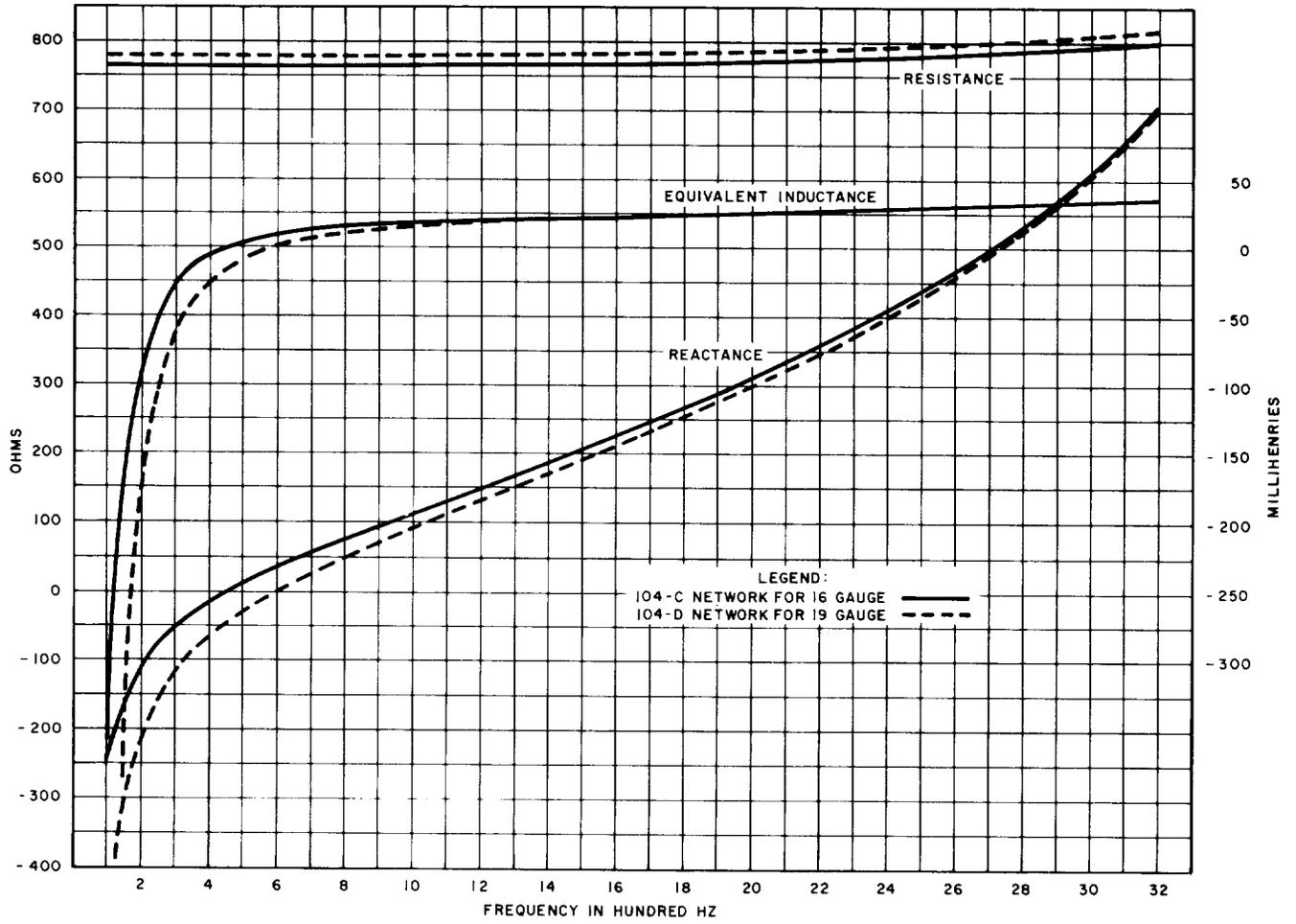
Fig. 8—Impedance of Networks for Toll Cable 104-Type Networks for H-63 Phantom Circuits
