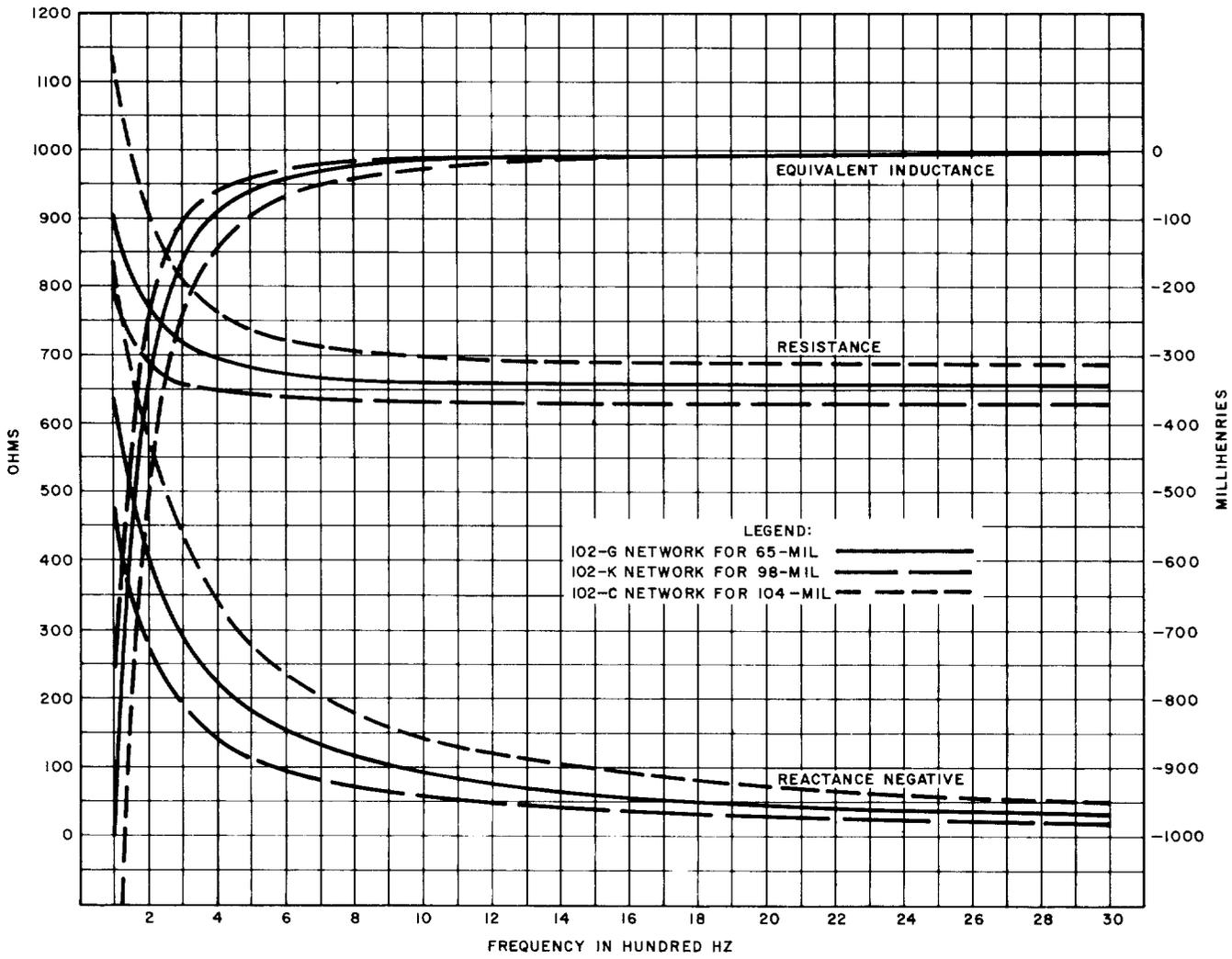
Fig. 3—Impedance of Networks for Nonloaded Open-Wire Circuits—102-Type Networks for Half-Pole Pair Side Circuits
