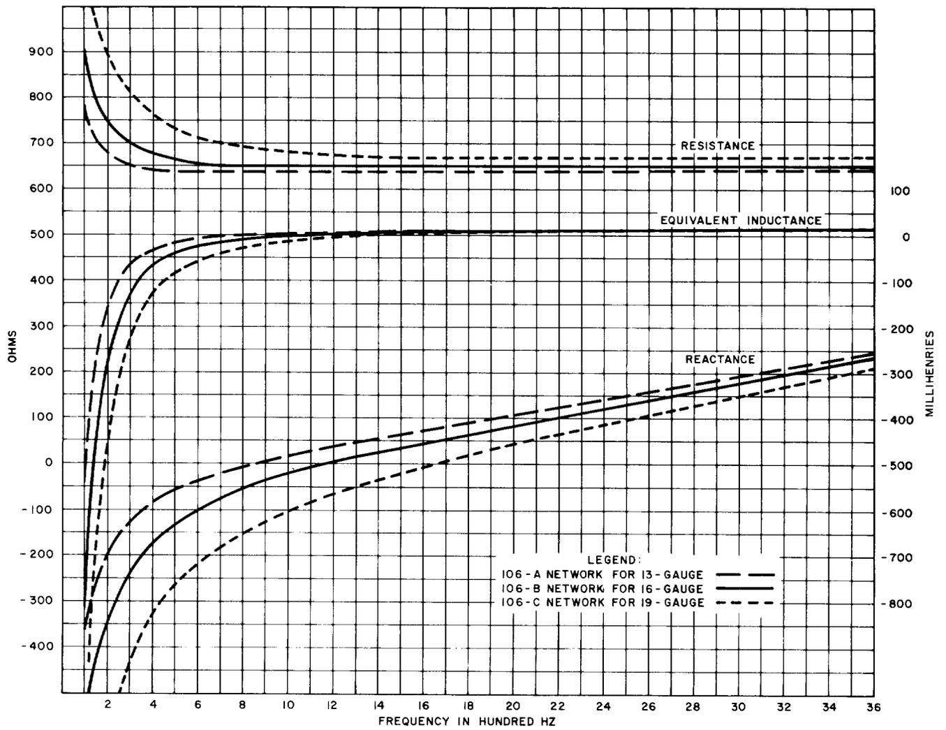
Fig. 12—Impedance of Networks for Toll Entrance Cable—106-Type Networks for H-28-16 Loaded Side Circuits
