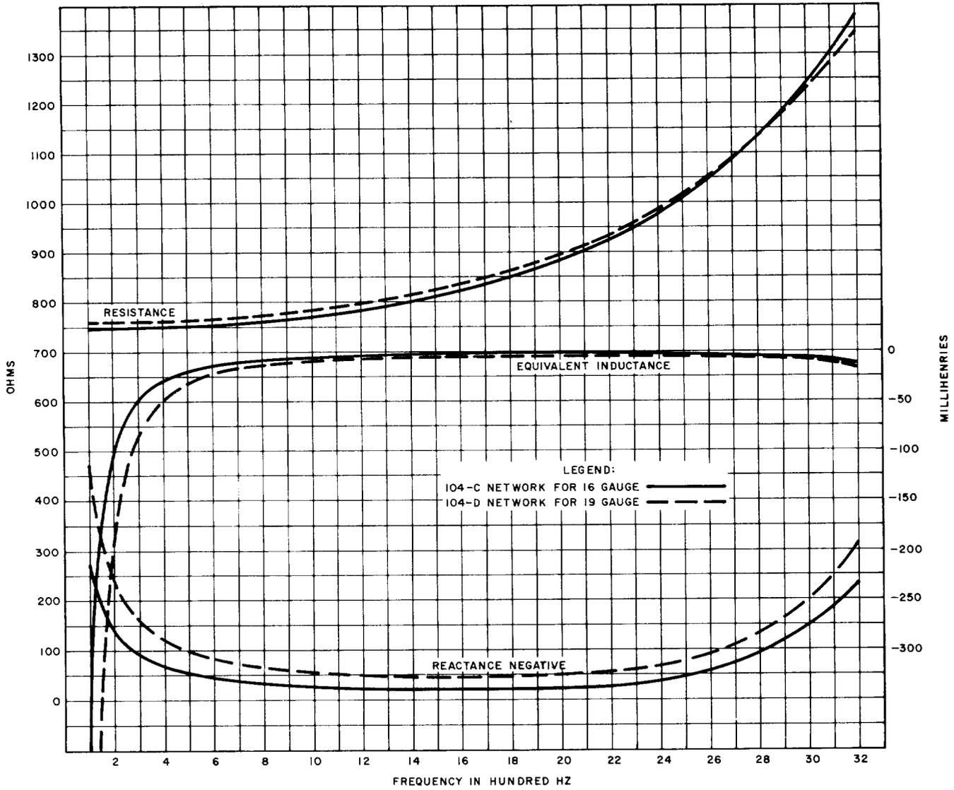
Fig. 7—Mid-Section Impedance of Networks for Toll Cable 104-Type Networks for H-63 Phantom Circuit
