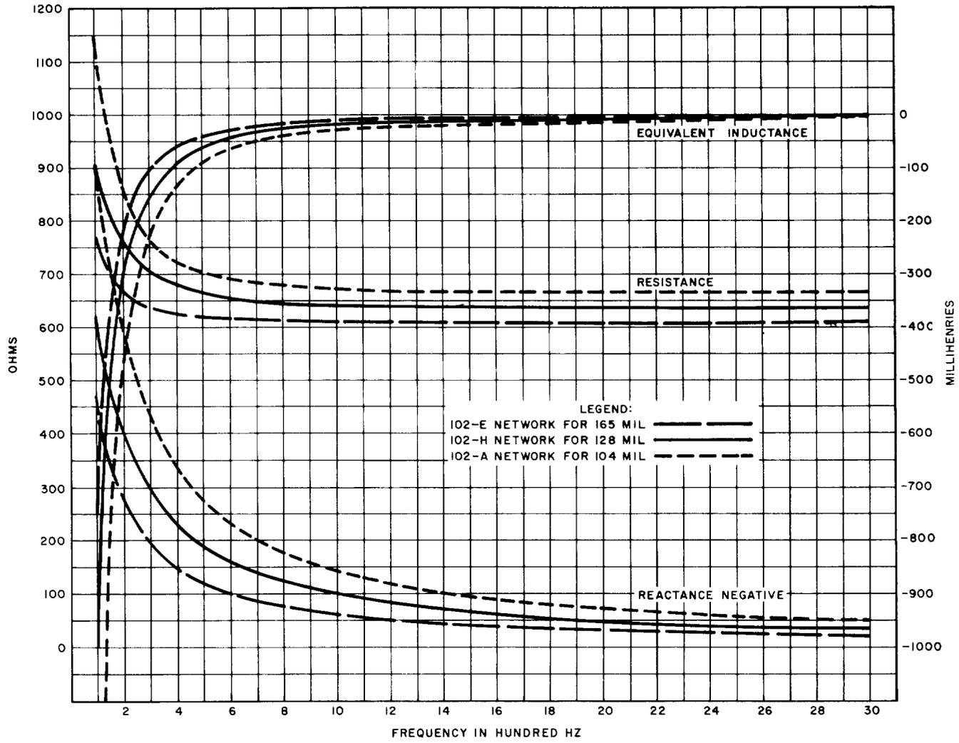
Fig. 1—Impedance of Networks for Nonloaded Open-Wire Circuits—102-Type Networks for 12-Inch Spaced Side Circuits
