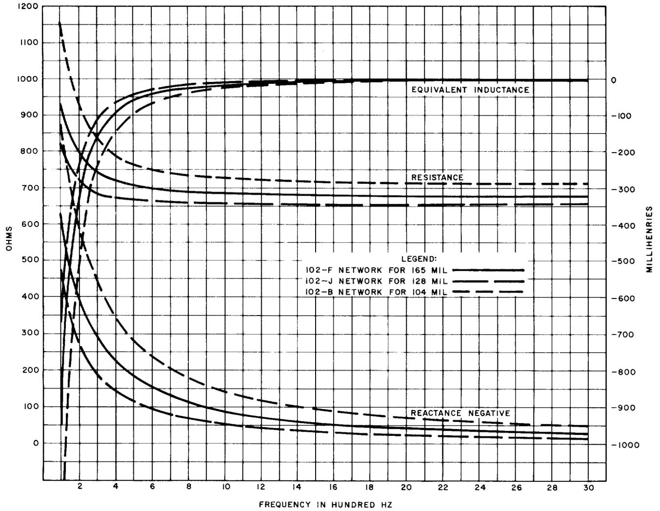
Fig. 2—Impedance of Networks for Nonloaded Open-Wire Circuits—102-Type Networks for Pole Pair Side Circuits
