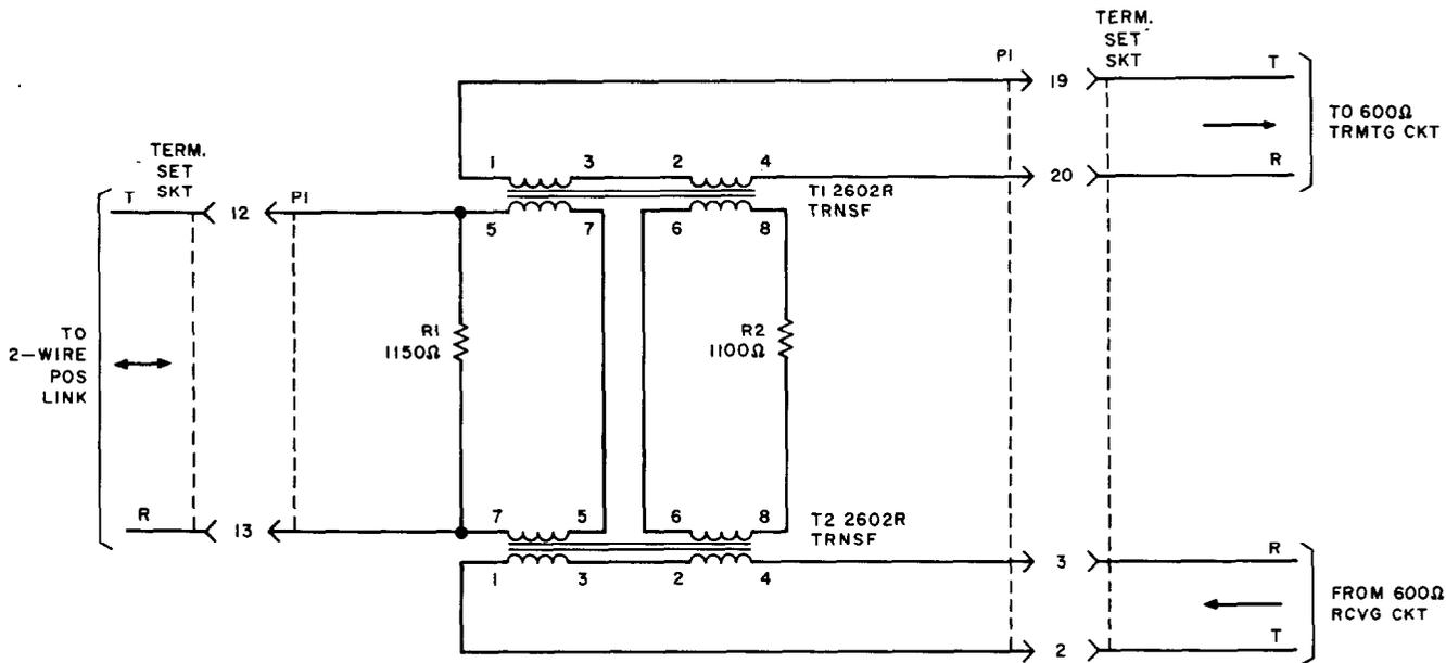
Fig. 2—1J Terminating Set—For Bridging on 600-Ohm 4-Wire Trunks—Schematic
