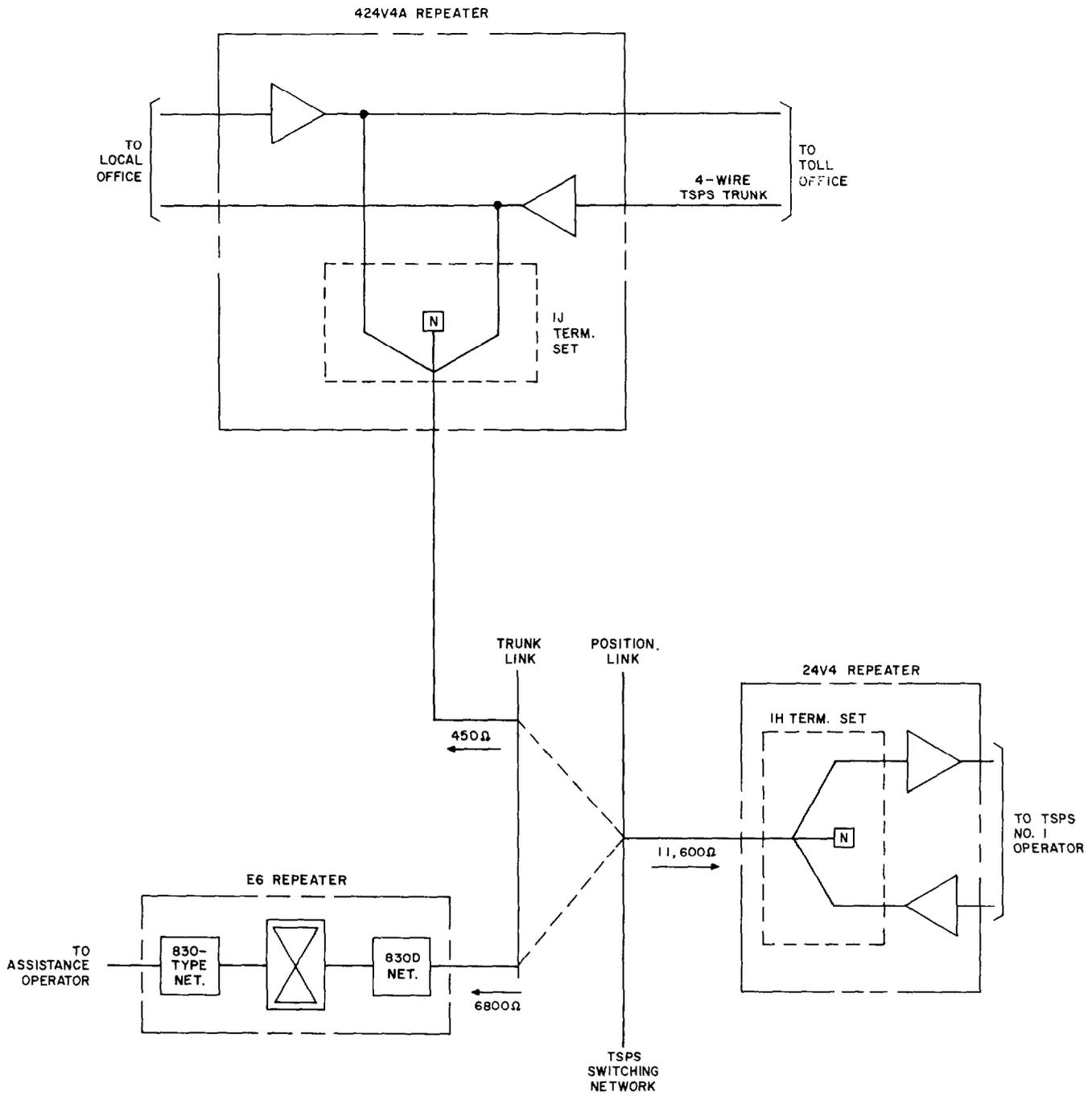
Fig. 3—TSPS No. 1 System—Block Diagram of Transmission Circuit
