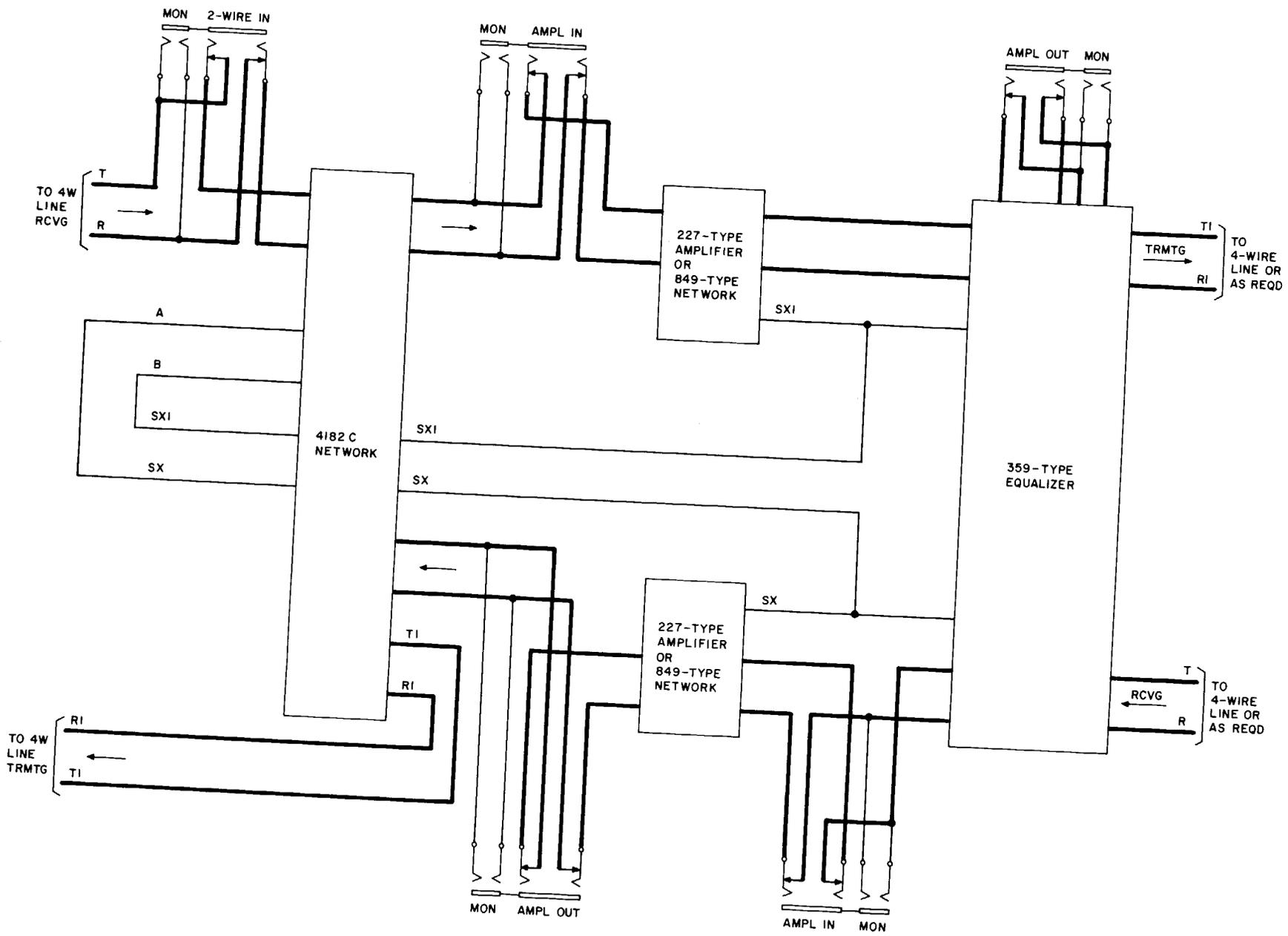
Fig. 12—4182C Network Used in 24V4 Repeater Mountings—No Signal Conversion Required
