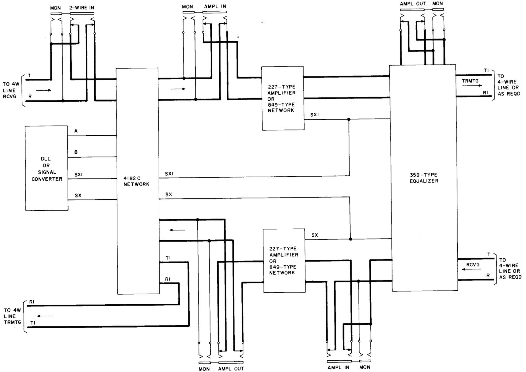
Fig. 13—4182C Network Used in 24V4 Repeater Mounting—Signal Conversion or Repeat Signal Required
