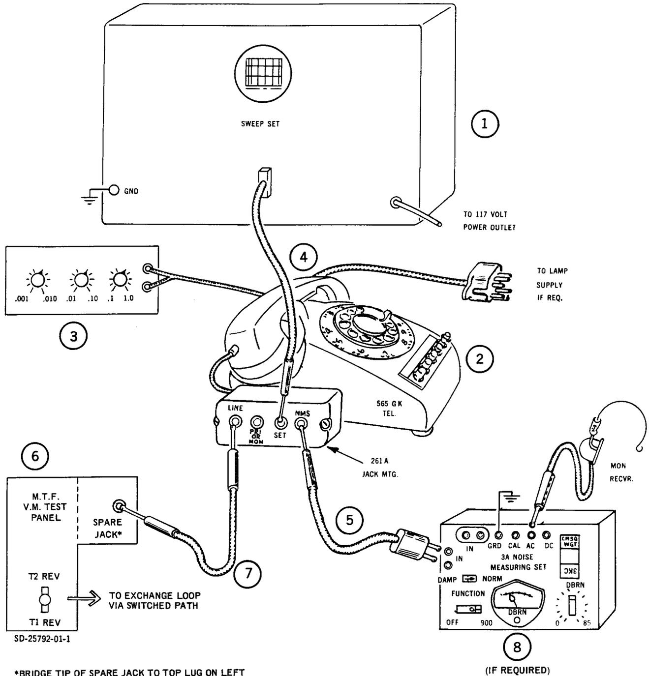
\*BRIDGE TIP OF SPARE JACK TO TOP LUG ON LEFT SIDE OF KEY (RED WIRE WITH WHITE MARKER) AT VM TEST PANEL
