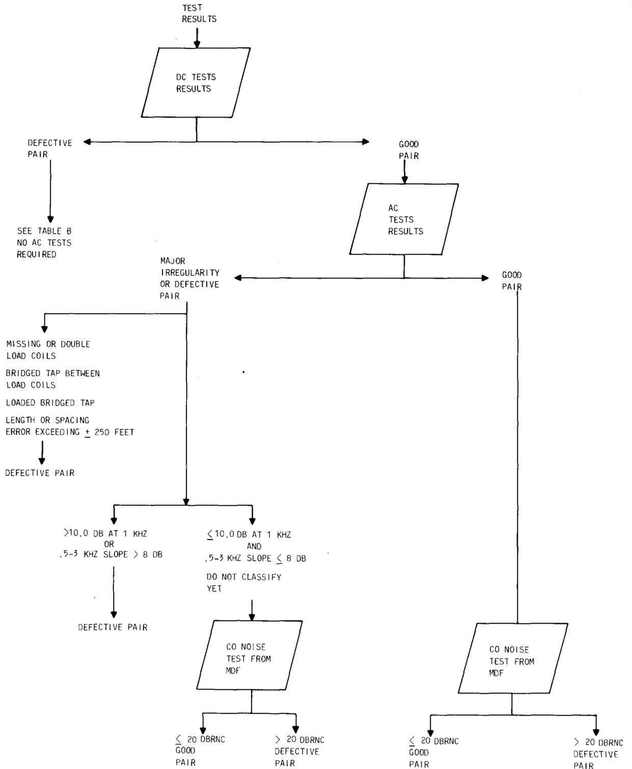
Fig. 1—Flowchart for Short Loaded Cables
