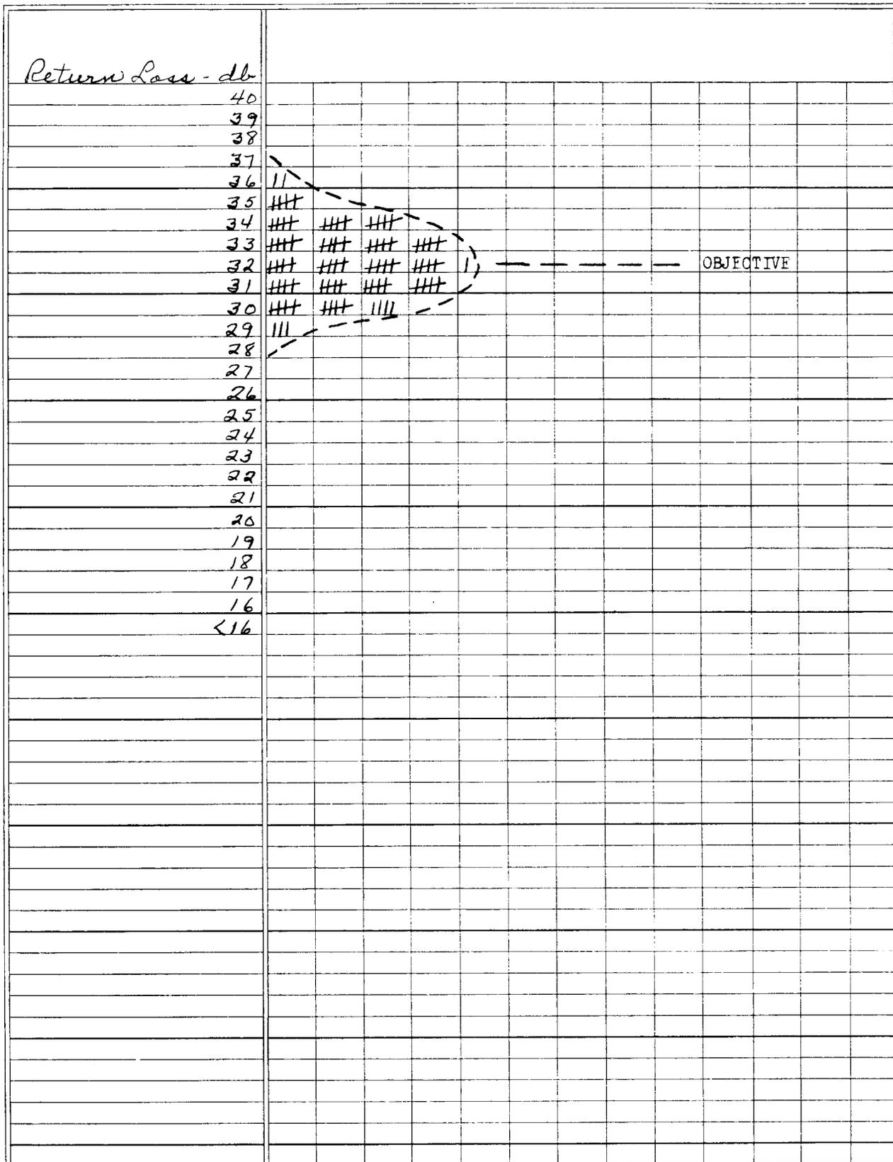
Fig. 1 - Tally of Return Losses — Complement of 100 Pairs
